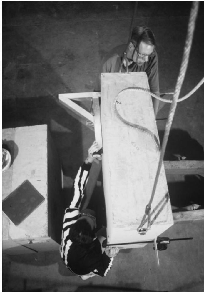
Figure 4.7: Erik Anderson and Jose Ortiz measure thickness sections for 305 mm nominal thickness plain concrete panel.
