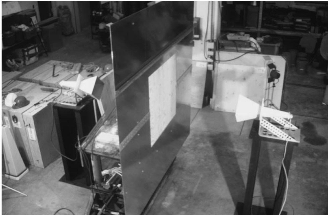
Figure 4.17: Test setup for specimen P50H (13 mm dry plywood panel) for frequency response determination from 3.0 to 8.0 GHz. See Figures 4.17c and 4.17d.
