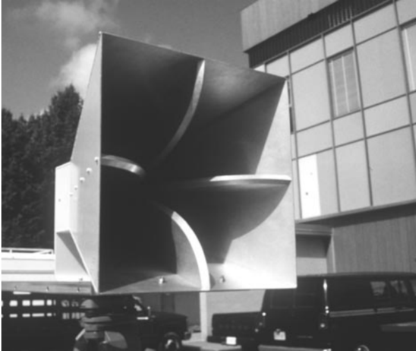
Figure 2.2.1: Quadridged 0.5 to 2.0 GHz . Vertical polarization, used for NIST tests, used only the two central vertical ridges.
