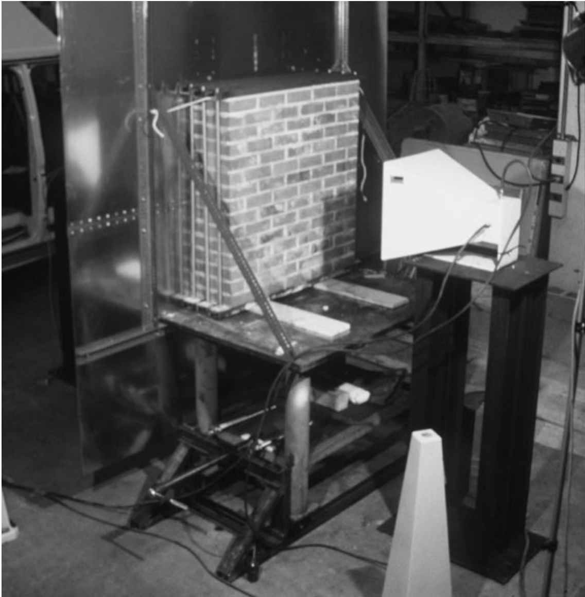
Figure 4.1: Test setup for specimen B3L (three-wythe deep brick wall) for frequency response determination from 0.5 to 2.0 GHz. See Figures 4.1a and 4.1b.
