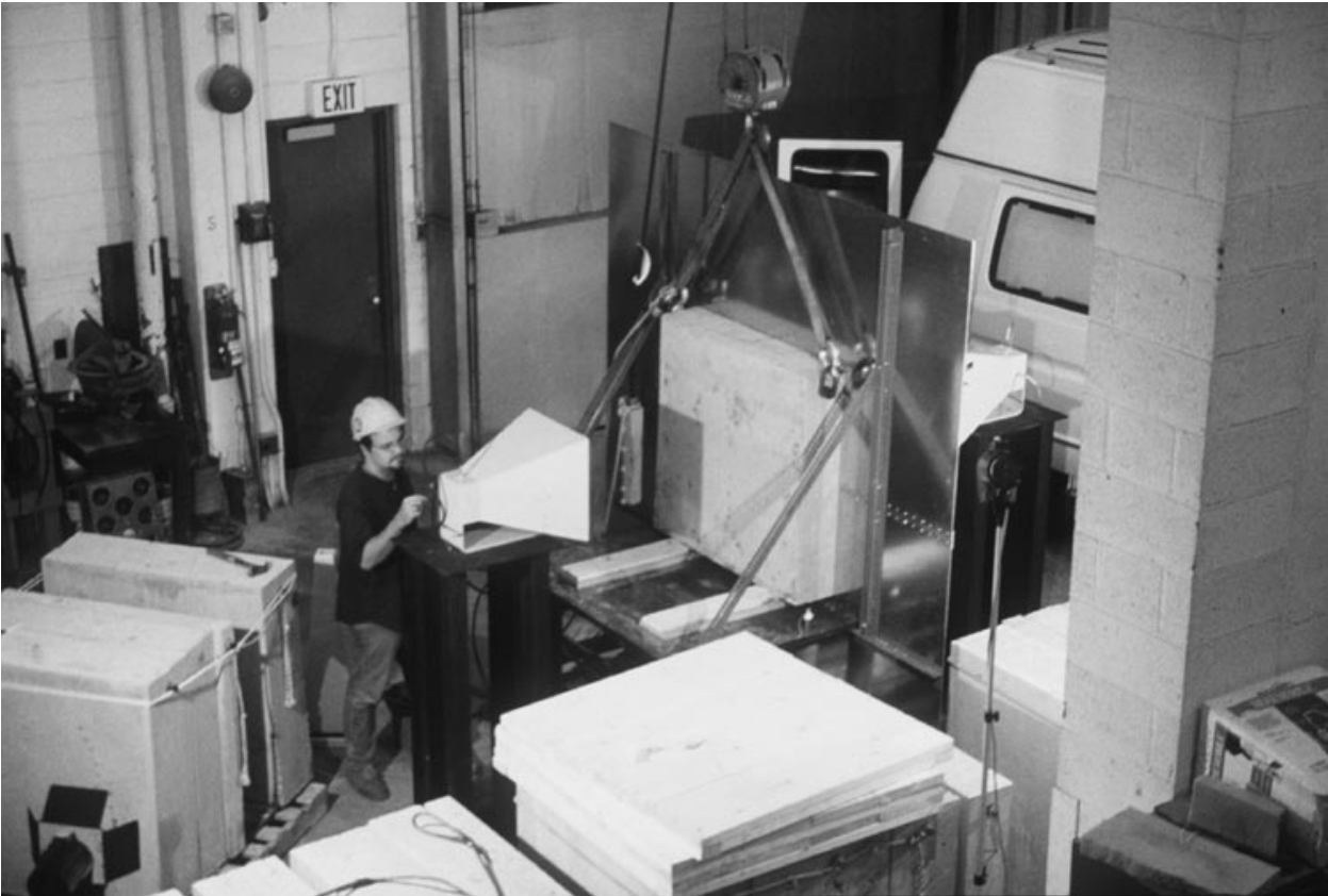
Figure 4.6: Adjusting low frequency (0.5 to 2.0 GHz) band receiver antenna for 203 mm concrete wall test.
