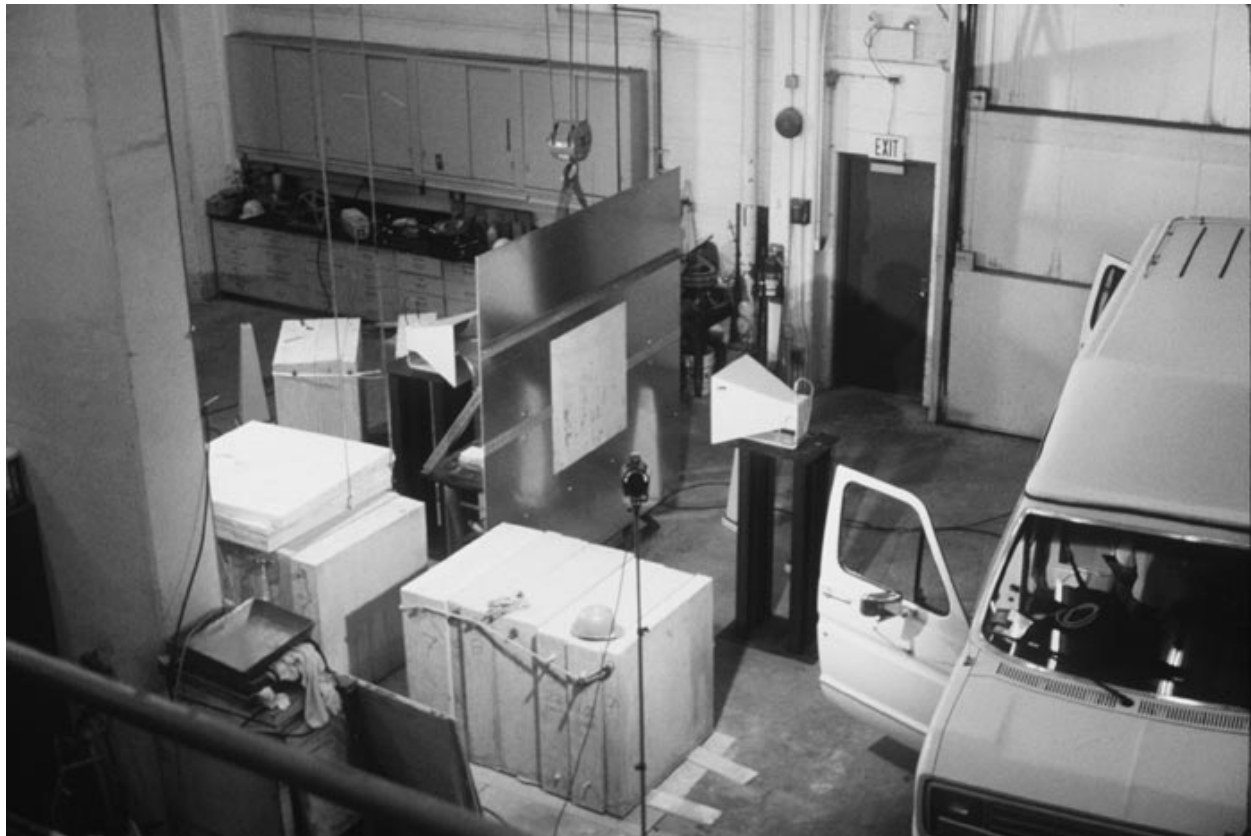
Figure 4.13: Test setup for specimen D25L (nominal 6 mm thick drywall panel) for frequency response determination from 0.5 to 2.0 GHz. See Figures 4.13a and 4.13b.
