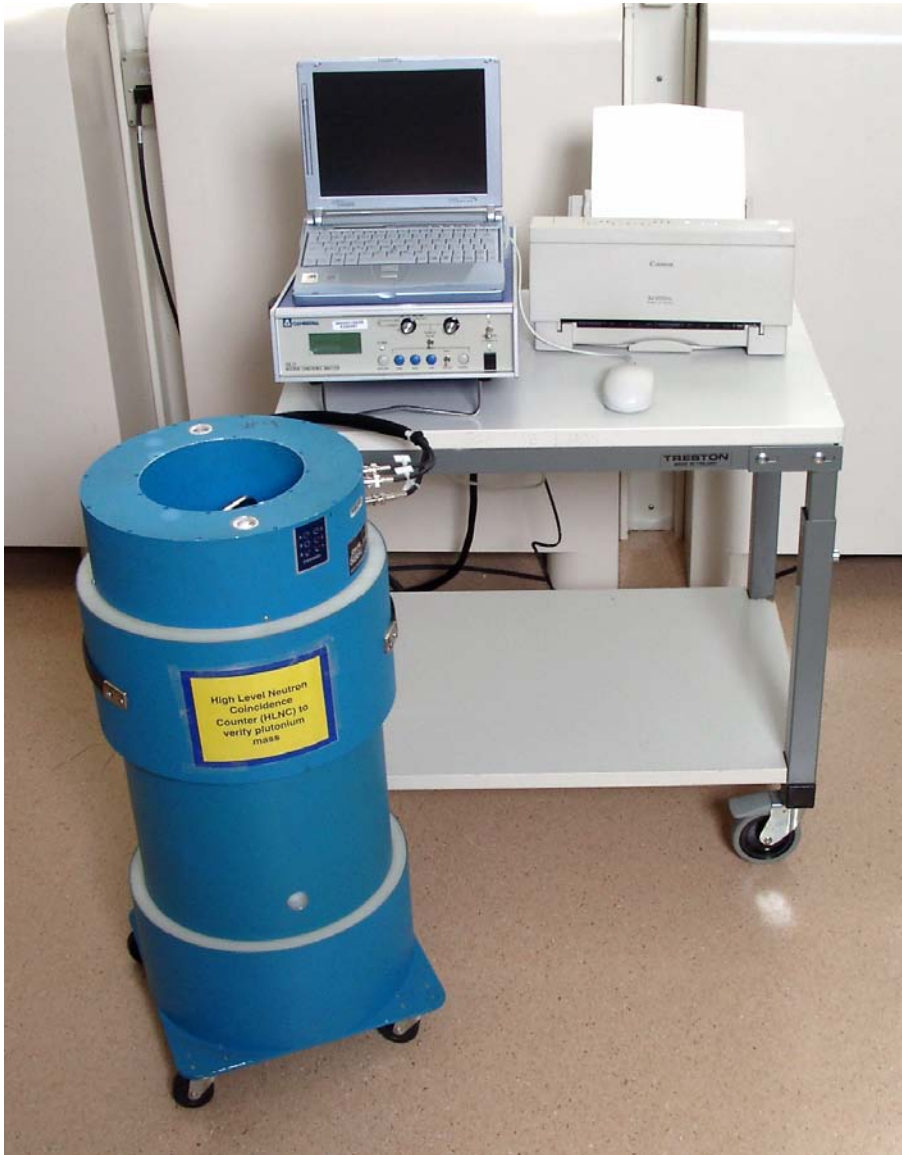
FIG. 7. High level neutron coincidence counter (HLNC).
