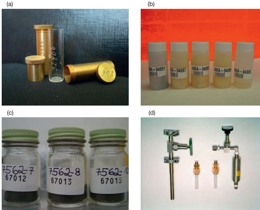
FIG. 45. Sample bottles used for IAEA verification samples: (a) vials for plutonium, MOX or high enriched uranium powder; (b) hard polyethylene bottle for hard or solid materials; (c) glass bottle for depleted, natural or low enriched uranium powder; (d) UF 6 container.
