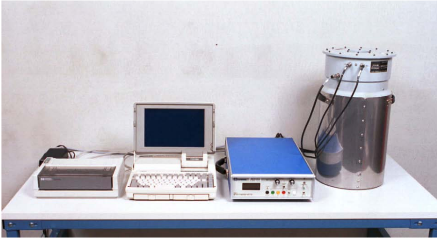
FIG. 8. Inventory sample (INVS) counter.
