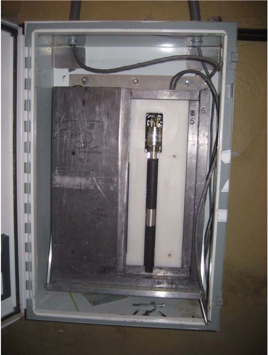
FIG. 20. Unattended spent fuel monitor (USFM).
