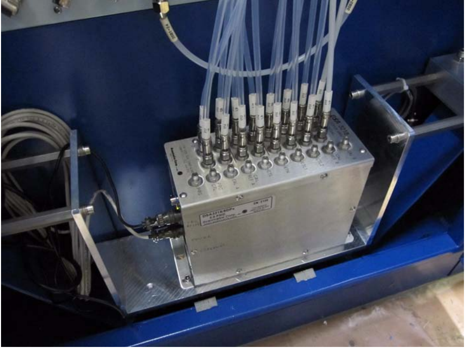
FIG. 24. Solution measurement and monitoring system (SMMS) pressure transducer.
