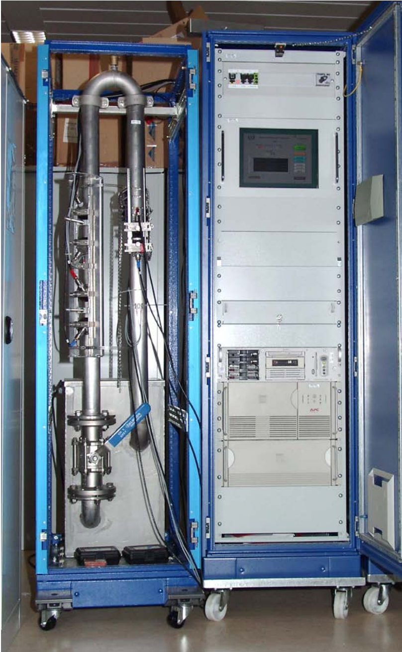
FIG. 23. Advanced thermohydraulic power monitor (ATPM).
