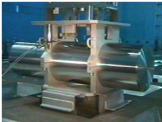
FIG. 12. Safeguards MOX python (SMOPY) device.
