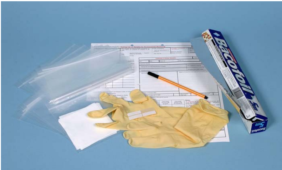
FIG. 55. Cotton swipe kit for environmental sampling.
