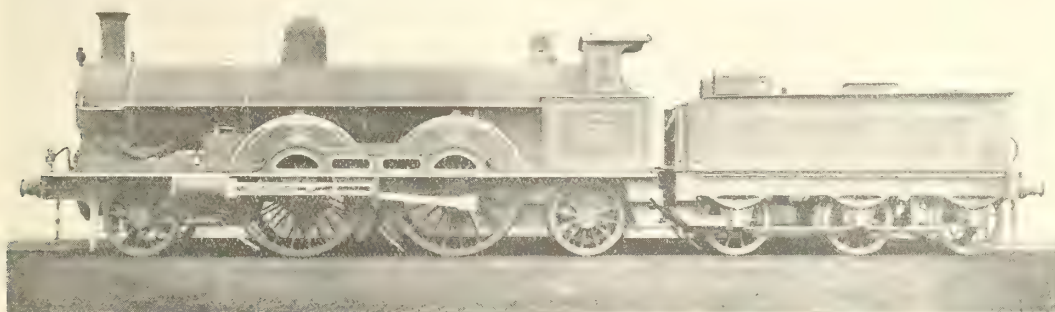
FIG. 365—F. W. WEBB'S THREE-CYLINDER COMPOUND ENGINE, "GREATER BRITAIN" CLASS, L. & N.W. RLY., 1891
