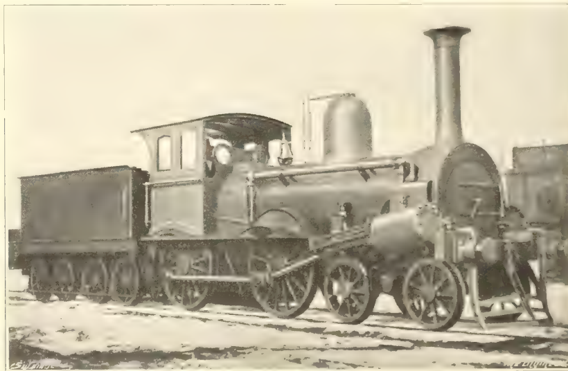
FIG. 171—KITSON'S ENGINE FOR THE COPIAPO & CALDERA RLY., CHILE, 1858
