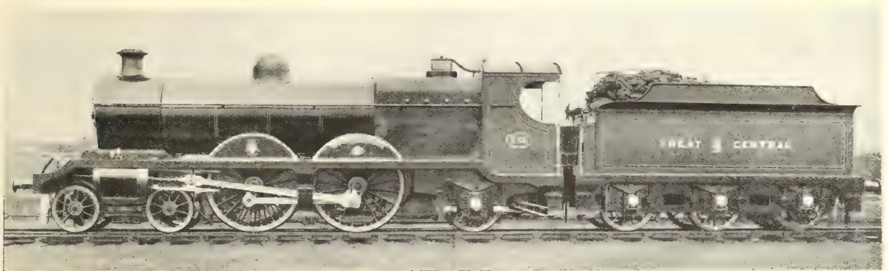
FIG. 405—J. G. ROBINSON'S THREE-CYLINDER COMPOUND EXPRESS LOCOMOTIVE, GREAT CENTRAL RLY., 1905
