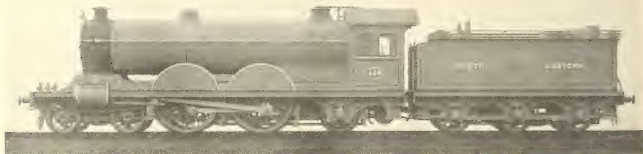
FIG. 417—W. WORSDELL'S "ATLANTIC" TYPE EXPRESS ENGINE, NORTH-EASTERN RLY., 1904
