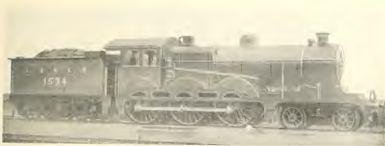
FIG. 419—S. D. HOLDEN'S 4-6-0 EXPRESS ENGINE, GREAT EASTERN RLY., 1911
