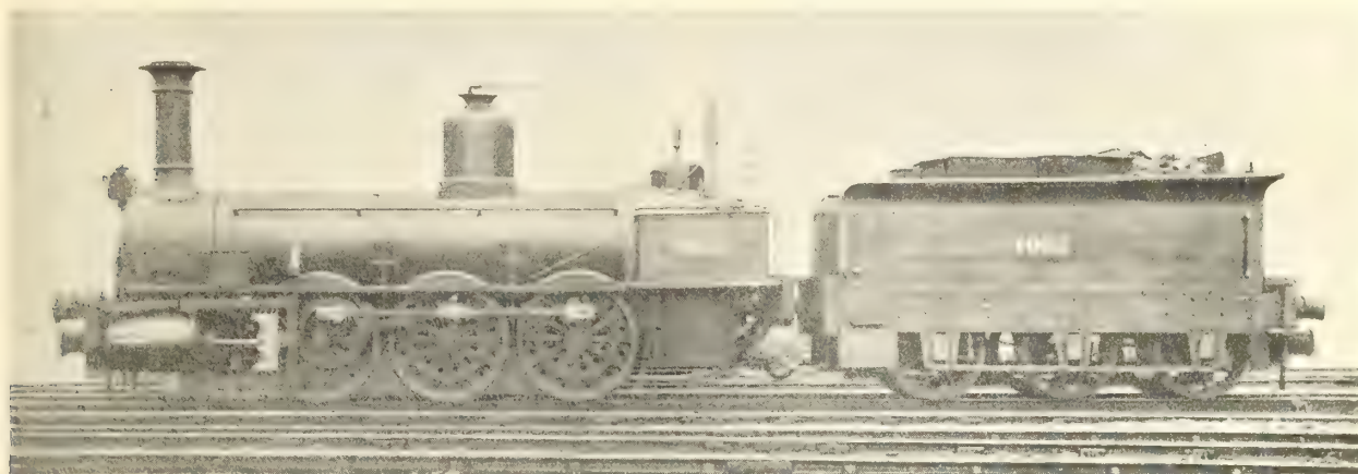
FIG. 63—W. BOUCH'S STOCKTON & DARLINGTON RLY. ENGINE "COMMERCE," BUILT AT SHILDON, 1847
