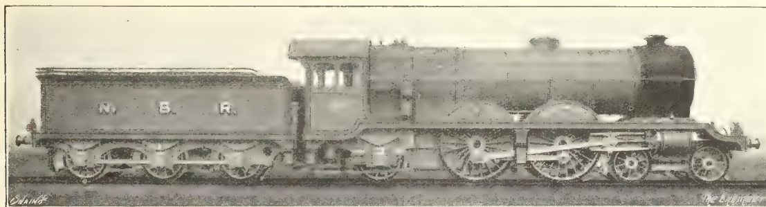
FIG. 416—W. P. REID'S "ATLANTIC" TYPE LOCOMOTIVE, NORTH BRITISH RLY. 1906-11
