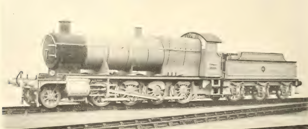
FIG. 443—G. J. CHURCHWARD'S EIGHT-COUPLED MINERAL ENGINE, GREAT WESTERN RLY., 1903
