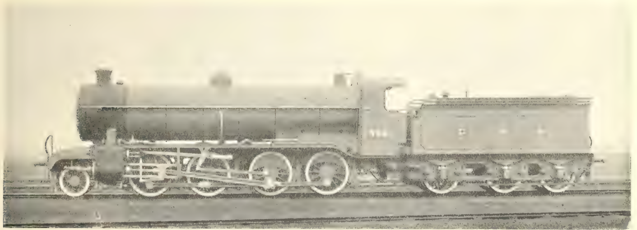
FIG. 445—H. N. GRESLEY'S 2-8-0 MINERAL TRAFFIC ENGINE, GREAT NORTHERN RLY., 1913
