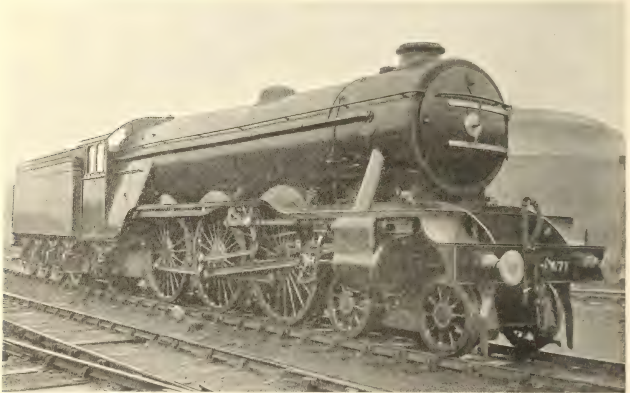
FIG. 457—H. N. GRESLEY'S THREE-CYLINDER "PACIFIC" TYPE EXPRESS ENGINE, GREAT NORTHERN RLY., 1922
