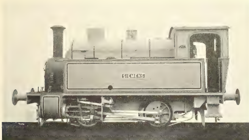
FIG. 448—BEYER, PEACOCK'S TANK ENGINE WITH BROTTAN WATER-TUBE FIRE-BOX, 1907
