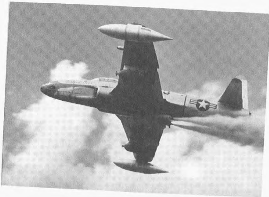
Above: A Lockheed F-80 Shooting Star fighter-bomber, using JATO take-off assistance rockets; below: When it first appeared, the MiG-15 posed a serious threat to U.N. air superiority.
