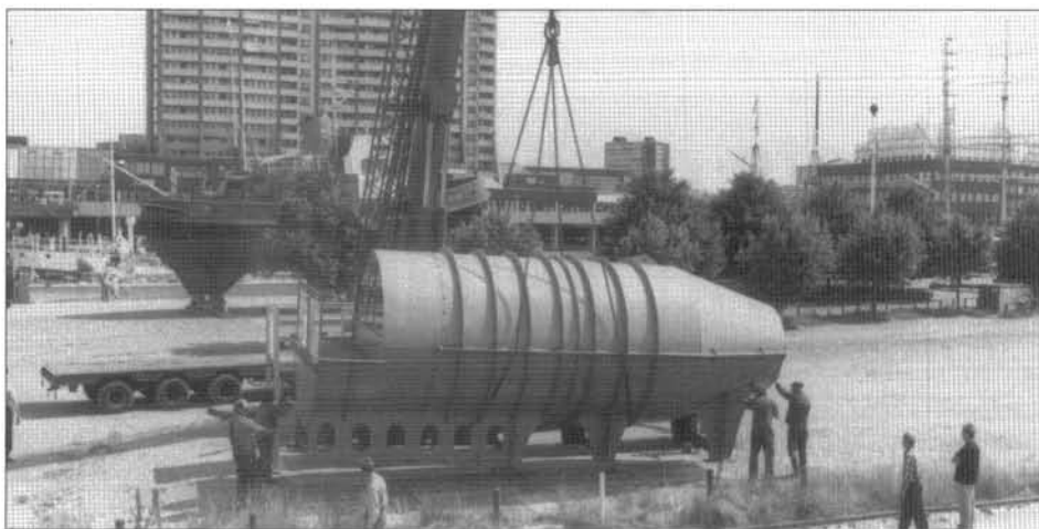
Right: The U-boat section containing the Walter turbine is lowered into position for display at the Deutsches Schifffahrtsmuseum.
