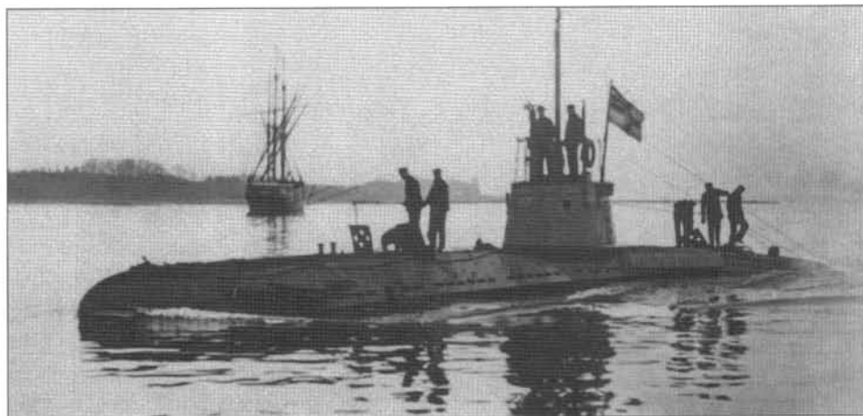
Right: UB 13, typifying the UB 1 class of coastal U-boat. This particular vessel was lost off Belgium in 1916.
