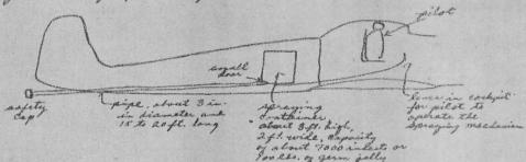
Spraying Mechanism in the Special aircraft
