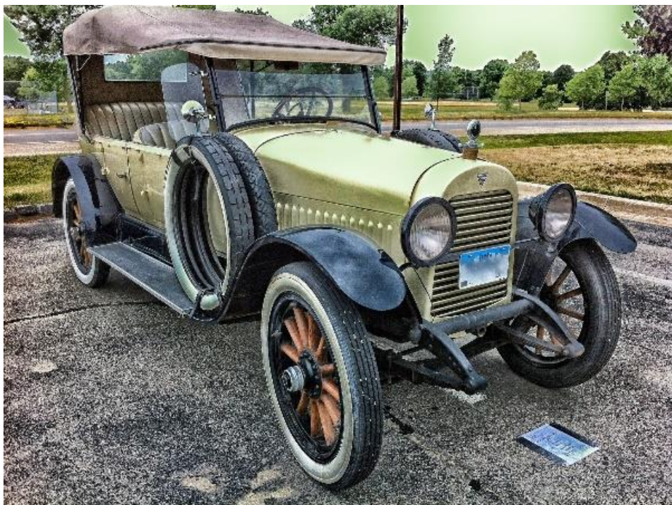
Figure 6.2. The 1921 Hudson Super Six Speedster Phaeton was powered by a 289 cubic-inch six-cylinder engine rated at 76 horsepower (57 kW). (Source: Image by David Mark from Pixabay)
