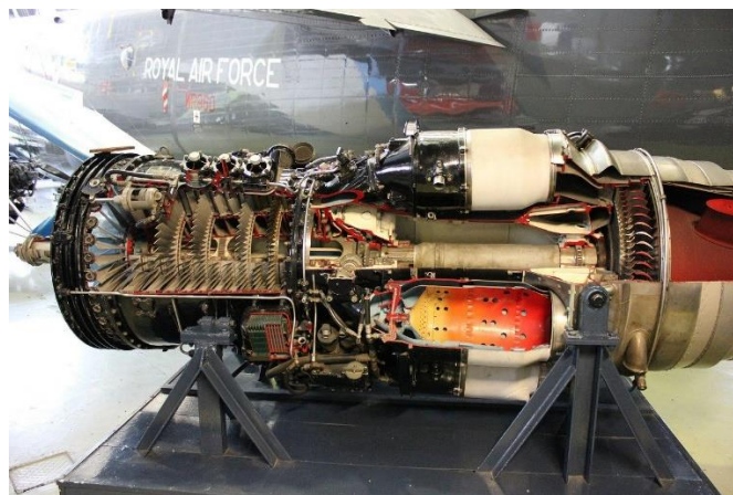
Figure 4.38. A cut away of a jet turbine (Image by PublicDomainPictures from Pixabay)
