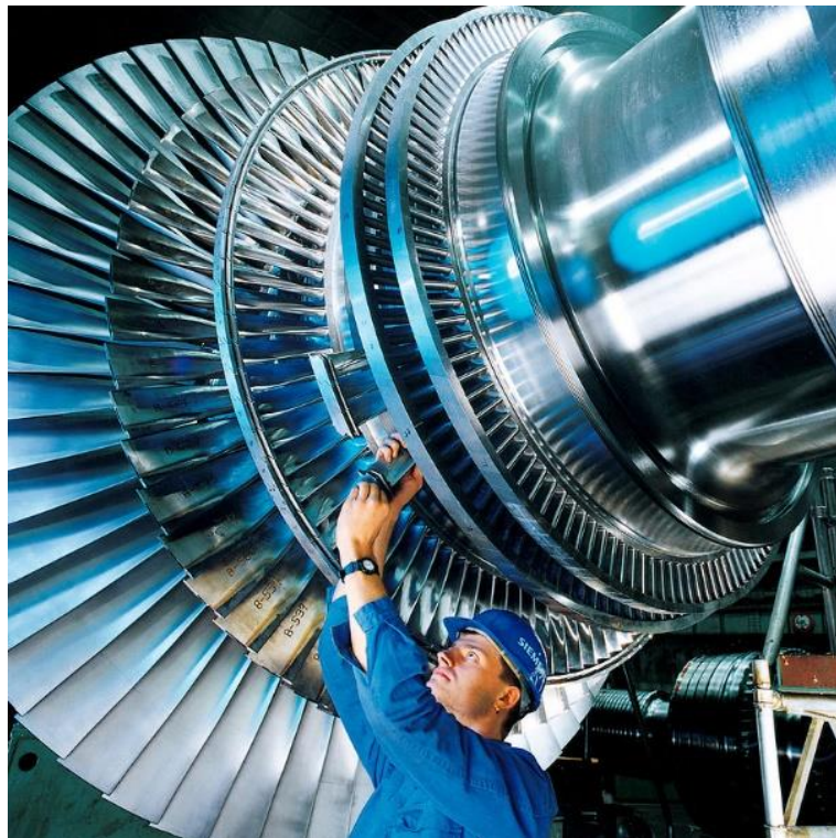
Figure 4.7. The rotor of a modern steam turbine used in a power plant
