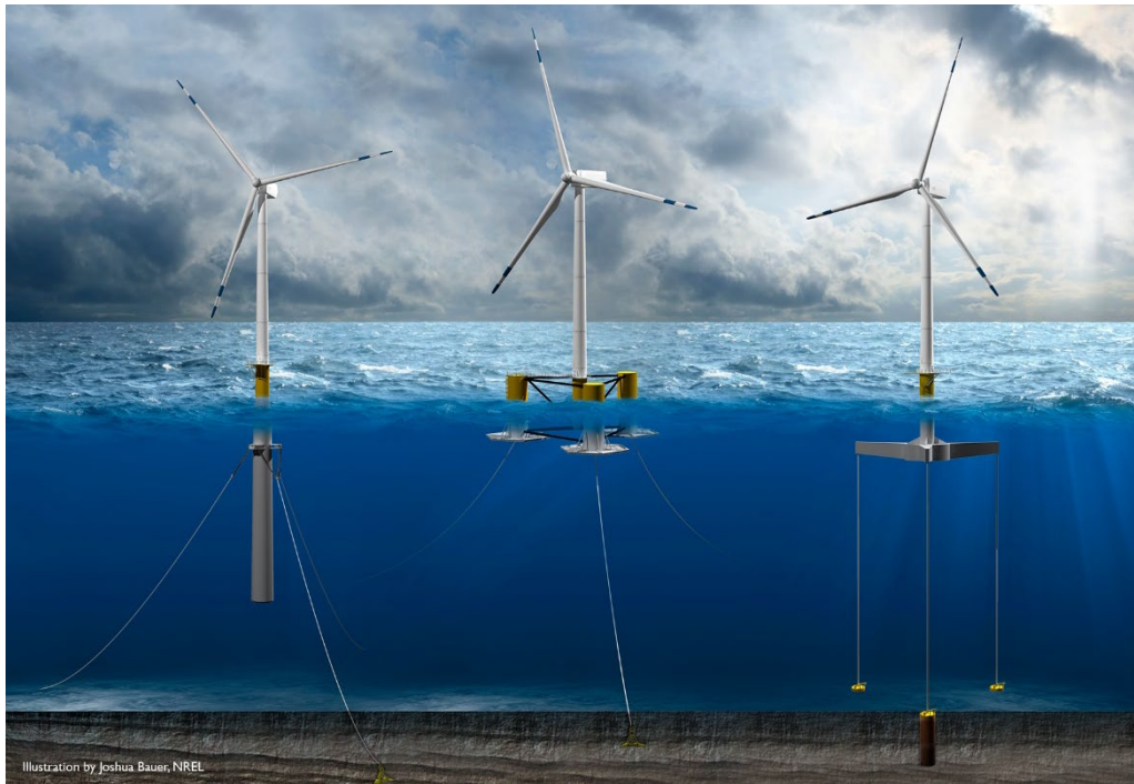
Figure 6-1 Illustration of key floating wind philosophies
