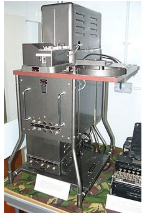
The Rockex was an IBM Telex machine adapted by Pat Bayly to operate on a one-time cypher, allowing secure communication among the Allies throughout the war. [20] It continued to be used in peacetime until the 1970s.
