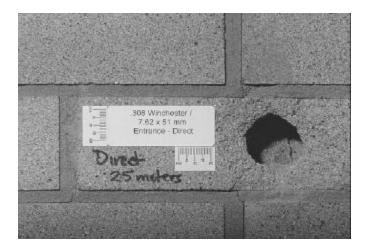
Figure 3 - Damage to clay brick caused by .308 Winchester
