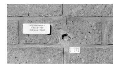
Figure 4 - Damage to concrete brick caused by .308 Winchester
