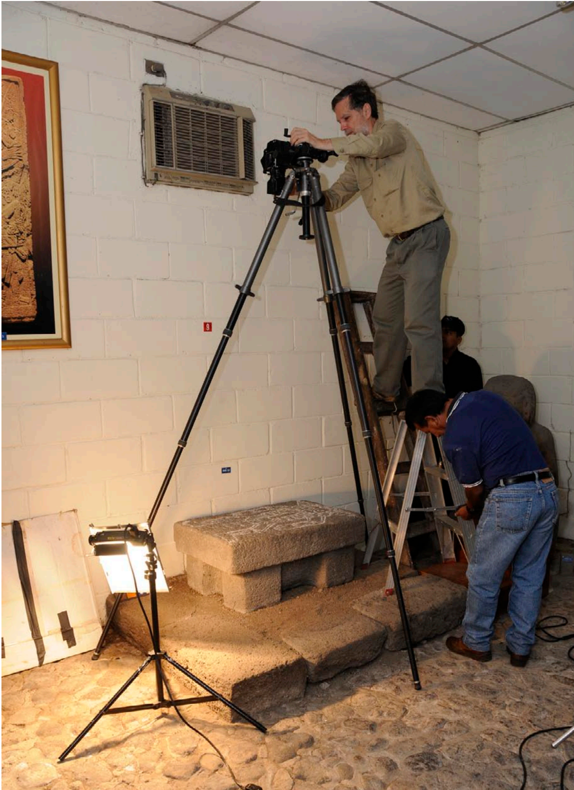
Figure 8. The Gitzo G1504 MK2 tripod can be raised 4 meters. In this photo you can see how usable the tripod is when you don't have a good angle of your object. Not many other brands or models of tripod can get your heavy camera safely directly over an object several meters below. Here you can see Dr. Nicholas Hellmuth trying to get his best shot on this situation.
