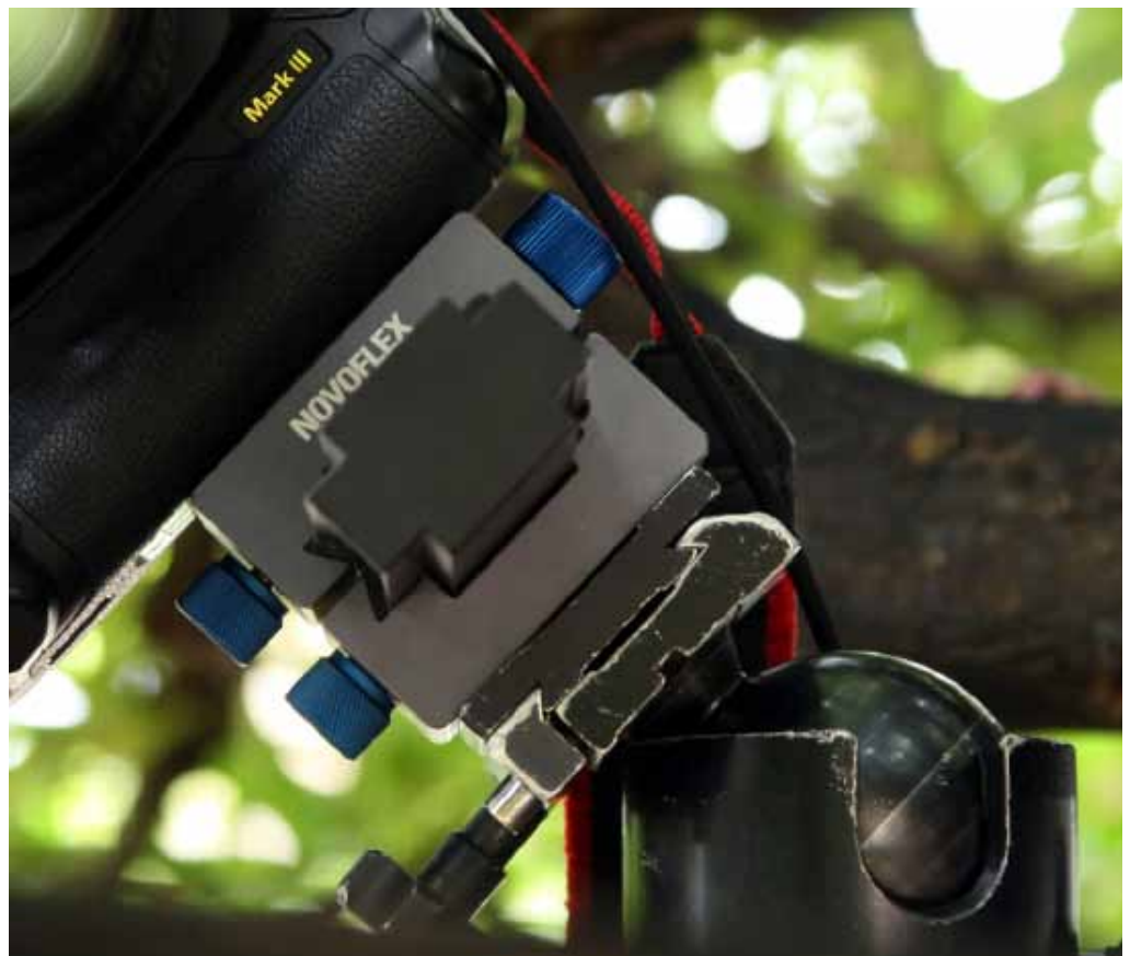
Canon EOS-1Ds Mark III atop a Novoflex focusing rack castel XL rail which is on an aging Arca-Swiss Monoball head, atop a Gitzo tripod.
