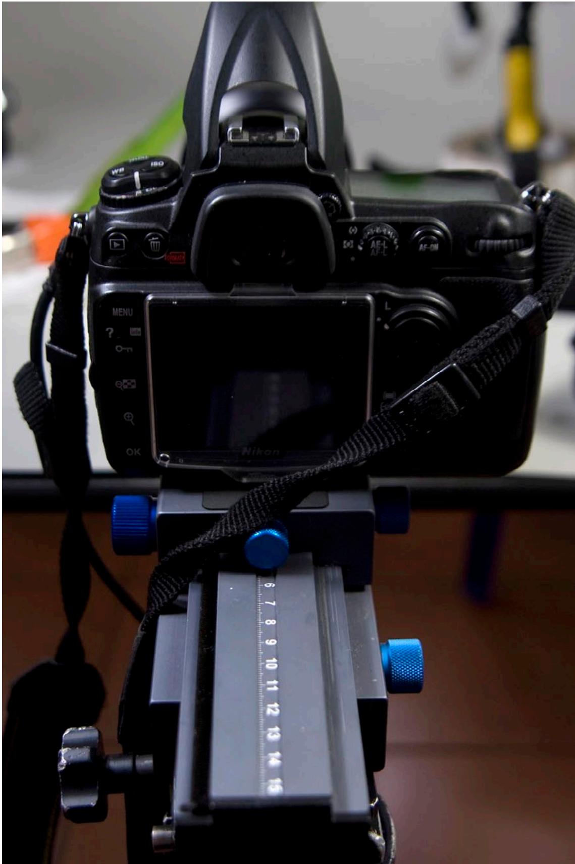
Figure 7. The Novoflex Castel-XL has numbers to help you keep track of where you are focusing when you are taking macro photographs.
