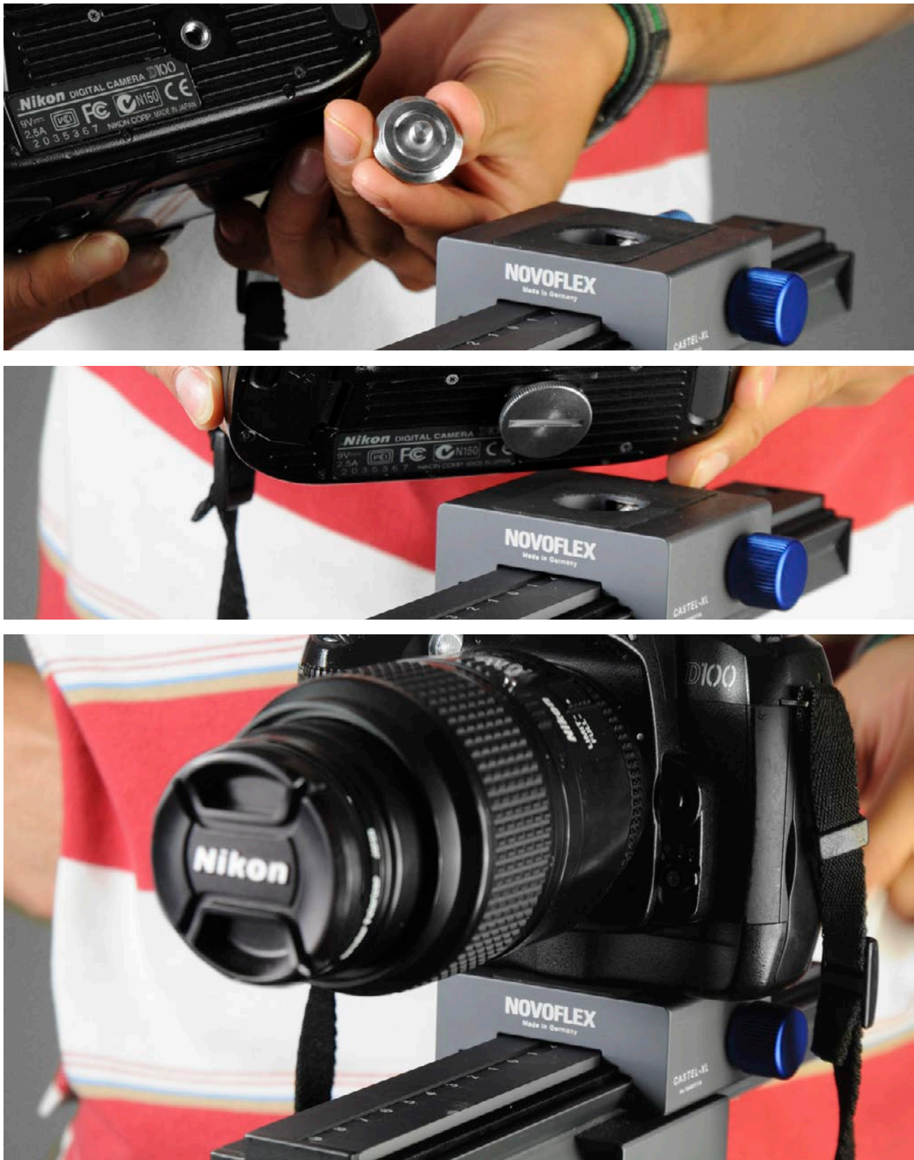
Figure 6. Here you can see the sequence of how to set up the camera in the Novoflex Castel-XL.
