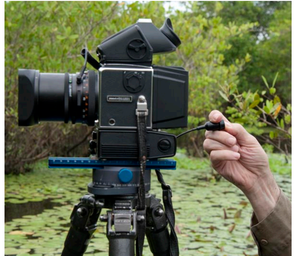
Be sure you use a cable release. We also trigger the mirror before we take the photo (in a single lens reflex, the mirror must flip out of the way before you take a photo. The movement of the mirror, and the clack! when it hits the resting point, are vibrations you don't want on your photo.
