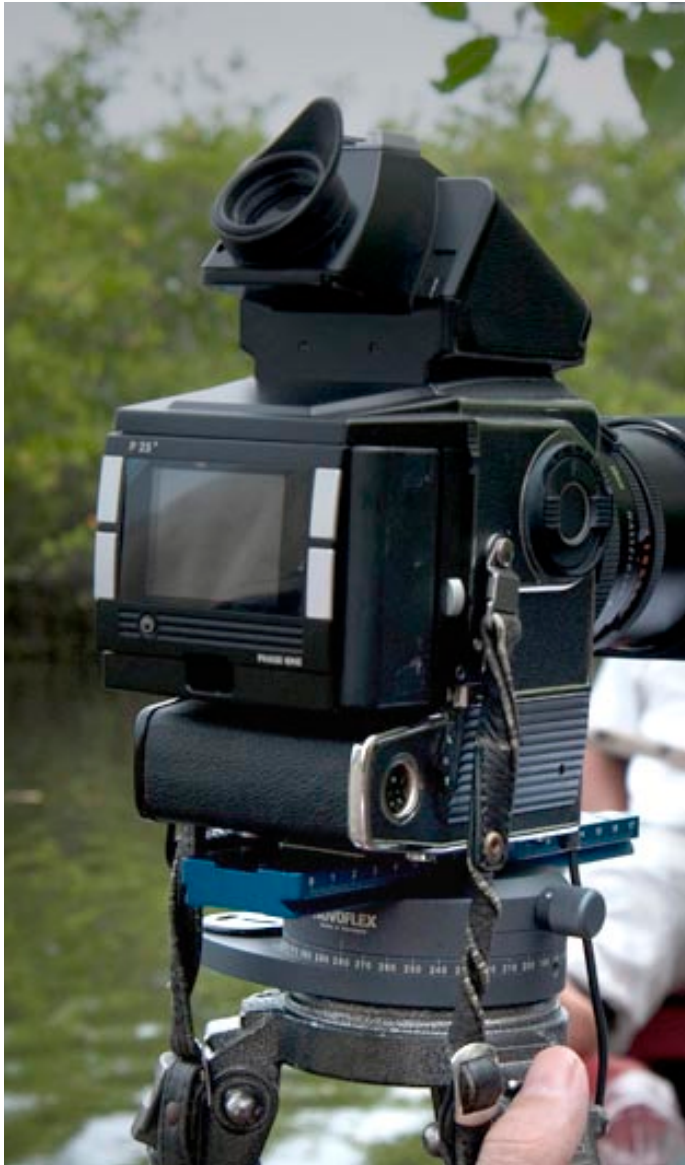
Now you can see the bulk and can imagine the weight of the medium format camera system. The digital portion is a Phase One P25+.
