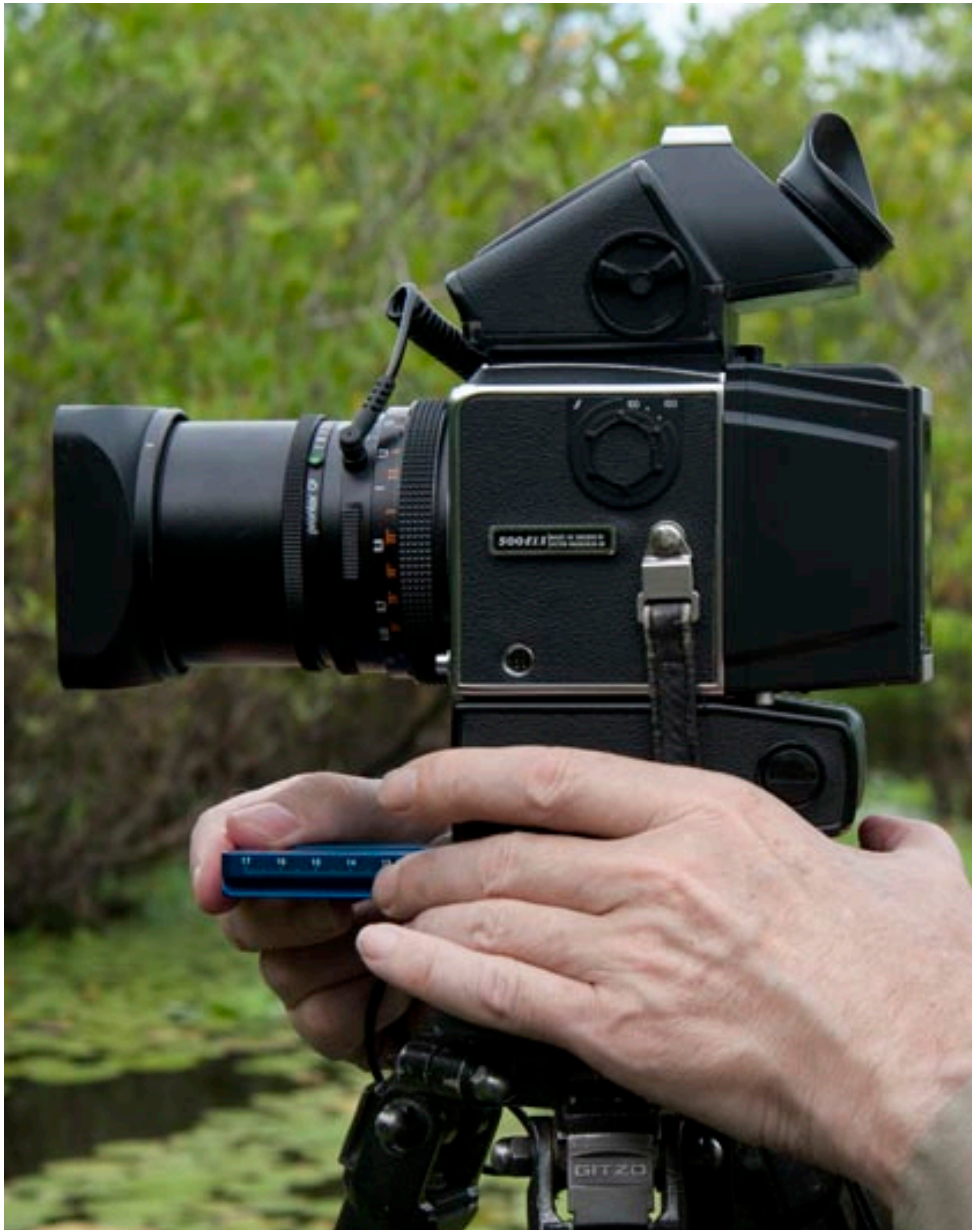
You can slide the base plate to a point where you find the nodal point.
