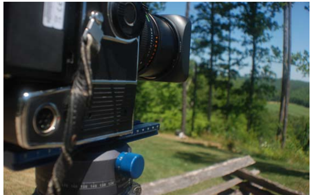
Here you can see the Hasselblad ELX, wide-angle 50mm Zeiss lens, lens shade, Novoflex PANORAMA=Q PRO. Not visible is the Gitzo tripod from Bogen. We are also interested in evaluating the QuadoPod from Novoflex but do not yet have one to test.
