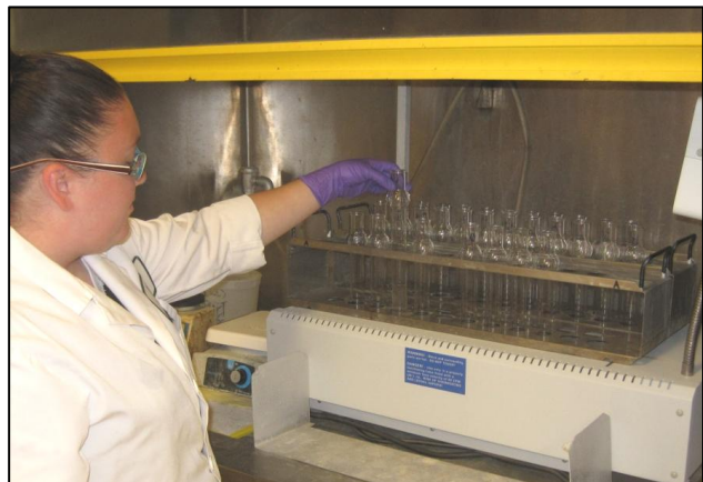
Total phosphorus analysis requires digestion before analysis, a step that is not necessary for orthophosphate.
