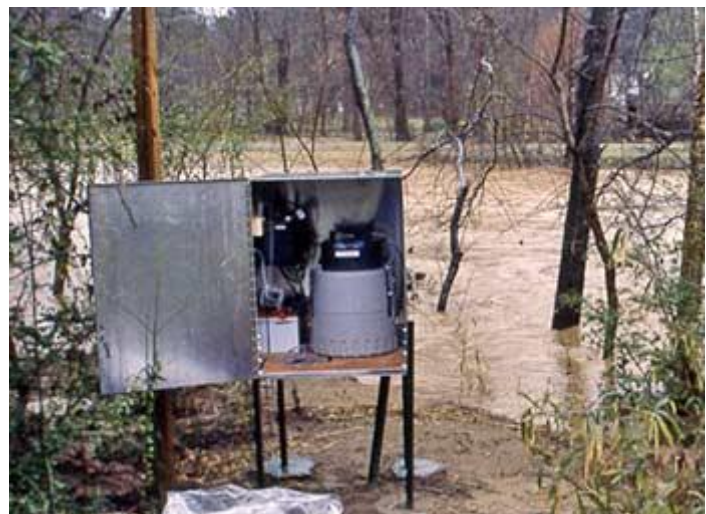
Figure T.1: Three methods for taking a sample. Top: Extended bottle holder. Middle: Simple dip and fill. Bottom: Automated sampler.
