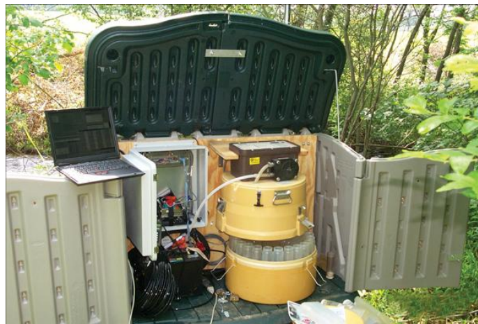
Automated sampling stations can collect samples at specific time intervals or proportional to flow over a specified period, greatly increasing the representativeness.
