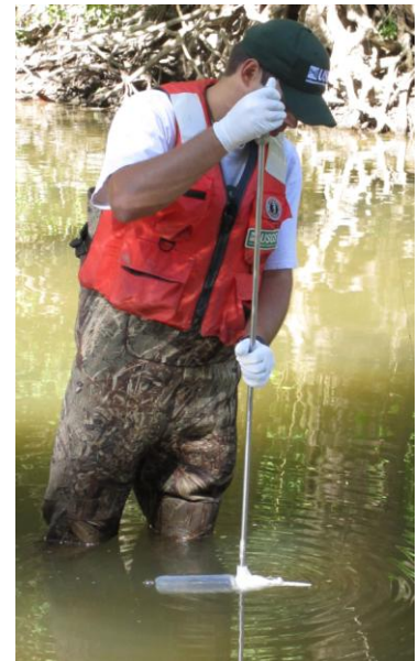
U.S. Geological Survey staff sampling the water column of a stream using a depth-integrating sampler.
