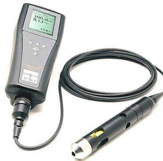
Dissolved oxygen is often measured with a digital probe.
