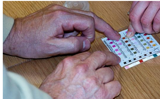
Volunteers match the color on the test strip to determine the pH level.
