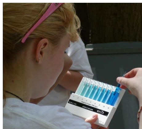
IDNR Hoosier Riverwatch volunteer analyzing DO using a test kit.
