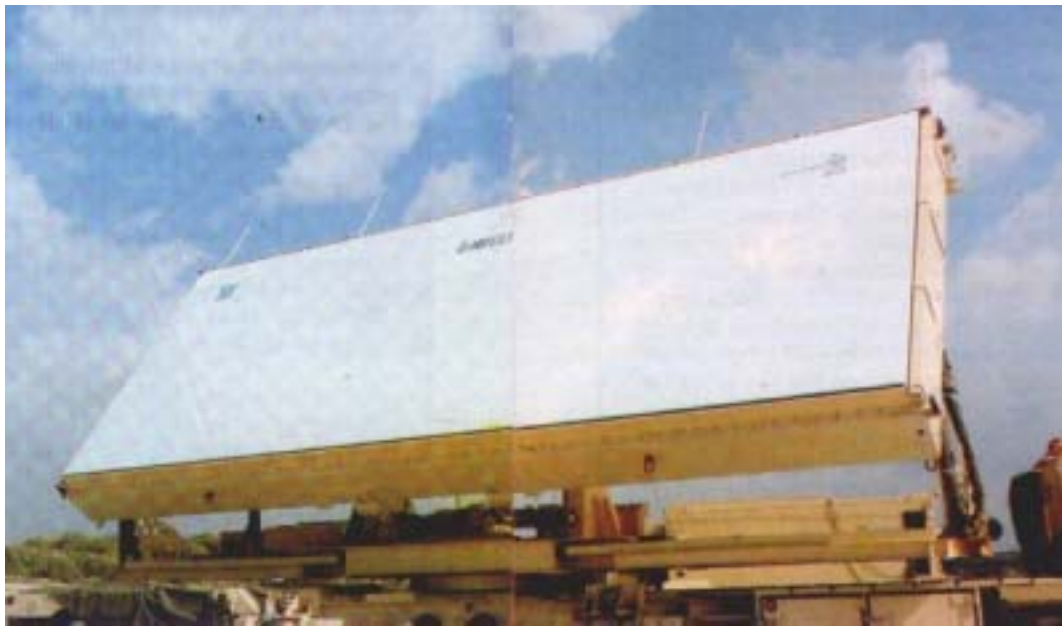
Figure 7 Elta L-Band EL/M-2080 Green Pine radar system: heart of the Arrow Weapon System (AWS) 35
