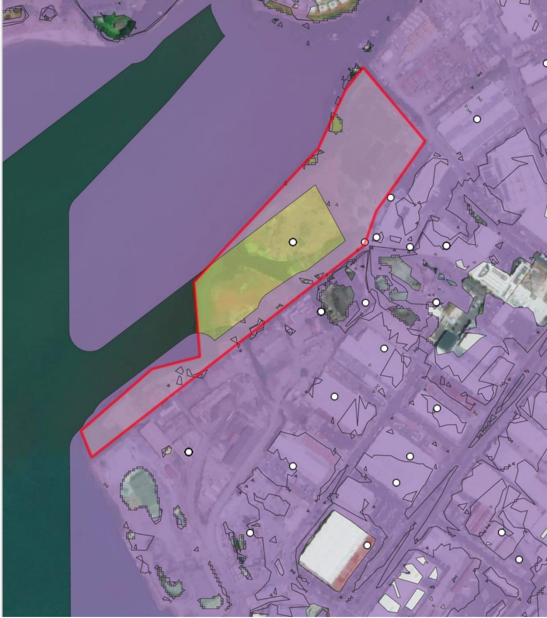
Figure 4: HEER site Keehi Lagoon Canoe Facility, Increment II in Honolulu Harbor (yellow area with red outline) in relationship to the area affected by 1% Annual-Chance Coastal Flood Zone in addition to 3.2 feet of SLR (purple).
