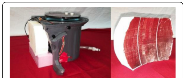
Fig. 156 (abstract A147). Left image showing imaging setup with mock transducer (white) radio-frequency coils (copper) phantom holder (gray) on the right is a mock transducer with 1x3 ground plane configuration
