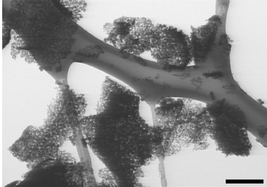
Supplementary Figure 4 | Low magnification SEM image of ZMO nanosheets obtained under 400 °C. Scale bar, 200 nm.
