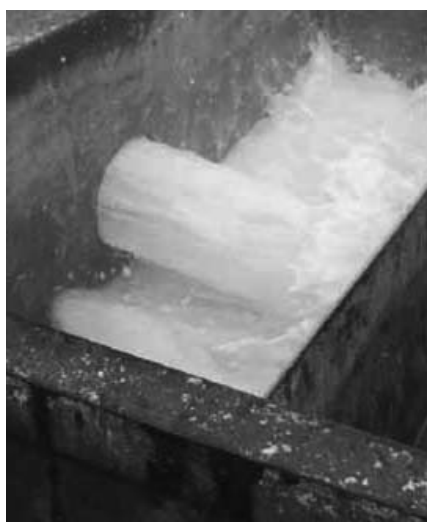
Warm water from almost 1,000m underground gushes up the borehole at a rate of 400 litres per minute into a tank, during geothermal exploration.
