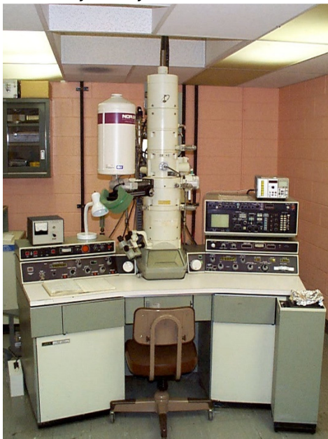
A Hitachi H-300 similar to the EMF microscope purchased by the Eye & Ear Institute
