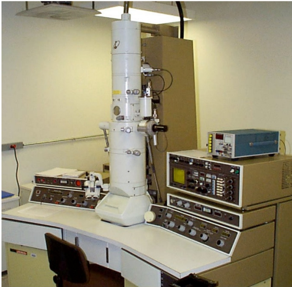
The JEOL JEM-100CX II 100kV TEM acquired from Civil & Materials Engineering (new 1986, EMS 1998-2015)
