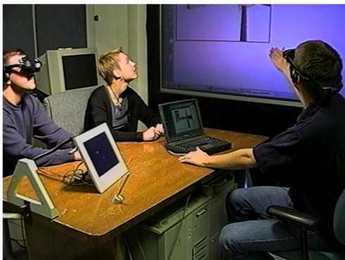
Figure 10: Heterogeneous displays in EMMIE, combining head-worn, projected, and private flat-screen displays. (Courtesy A. Butz, T. Höllerer, S. Feiner, B. MacIntyre, C. Beshers, Columbia University.)
