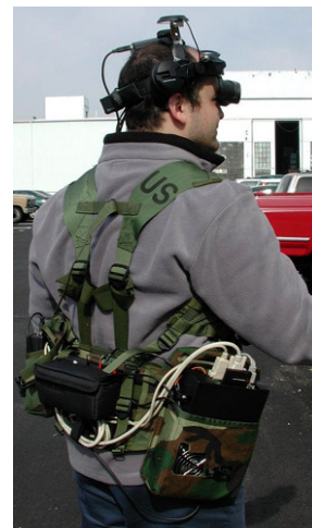
Figure 14: Battlefield Augmented Reality System, a descendant of the Touring Machine. (Courtesy Naval Research Lab, Columbia University.)
