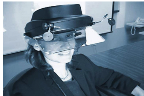
Figure 4: Experimental head-worn projective display using lightweight optics. (Courtesy of Jannick Rolland,
