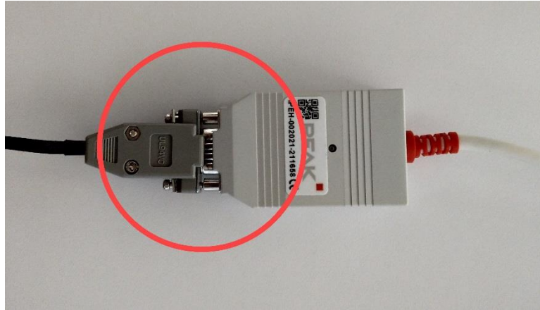
Figure 26. Connecting the EDR retrieval cable to the PCAN
