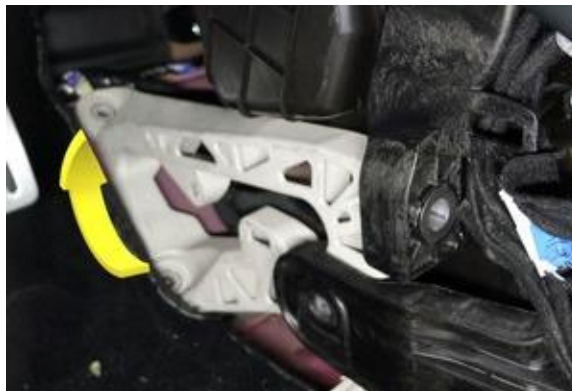
Figure 21. Removing the toeboard bracket from the vehicle
