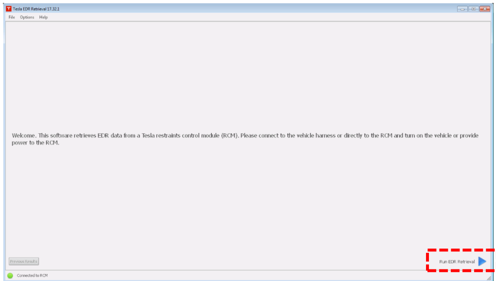
Figure 52. Retrieving data using the Tesla EDR retrieval program
