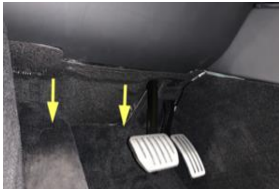
Figure 32. Removing the LH footwell cover
