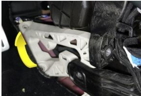
Figure 37. Removing the toeboard bracket from the vehicle
