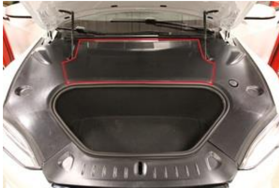
Figure 11. Removing the underhood apron
