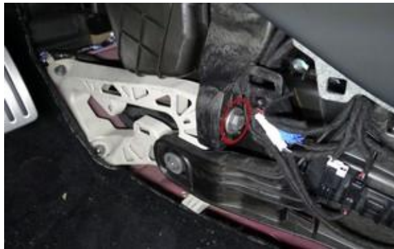
Figure 20. Releasing the toeboard bracket from the IP carrier
