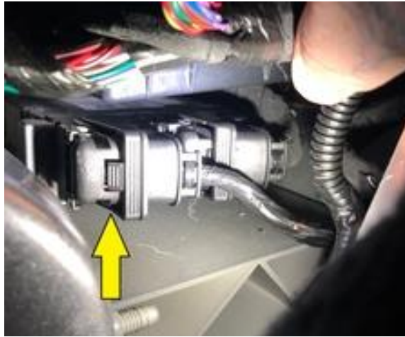
Figure 38. Disconnect the RCM connectors
