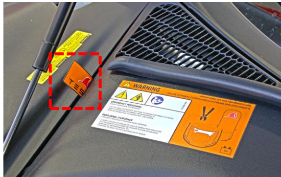
Figure 47. Opening the first responder access panel
