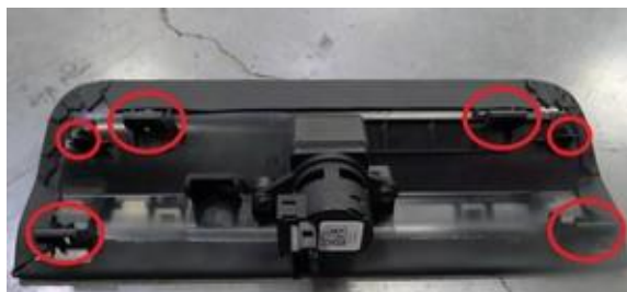
Figure 5. Removing the IP service panel
