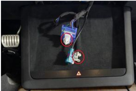
Figure 7. Releasing the diagnostic and CAN harnesses
