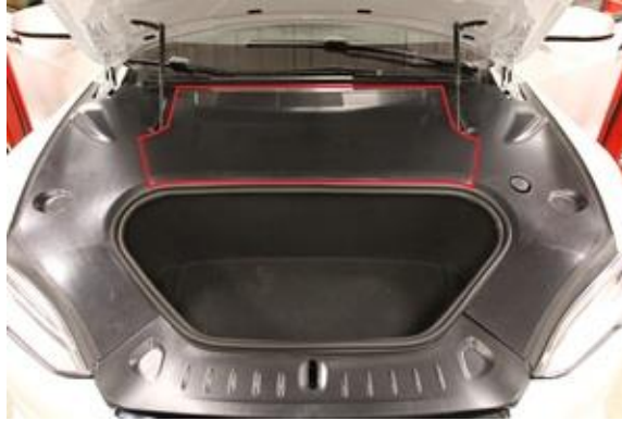
Figure 27. Removing the underhood apron
