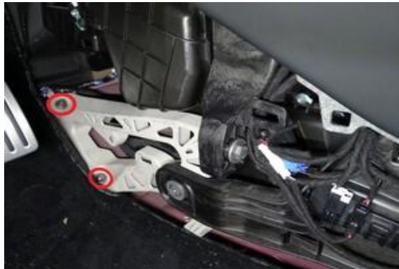
Figure 34. Releasing the toeboard bracket from the body
