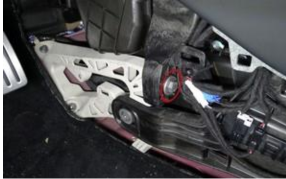
Figure 36. Releasing the toeboard bracket from the IP carrier
