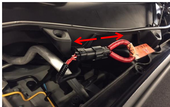
Figure 49. Disconnecting the first responder loop harness
