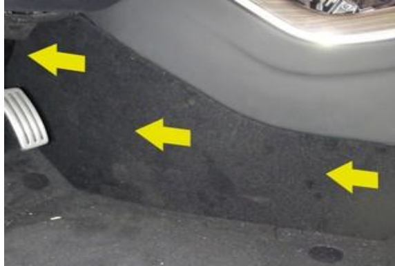
Figure 33. Removing the console side carpet
