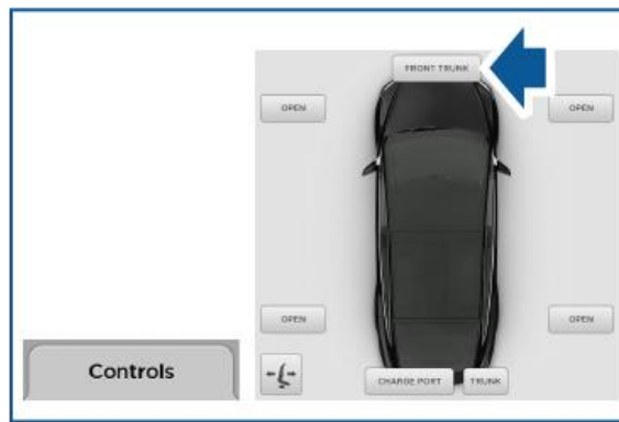
Figure 45. Opening the frunk using the touchscreen
