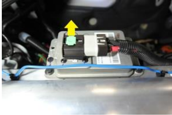
Figure 13. Unlocking the 12V battery connector
