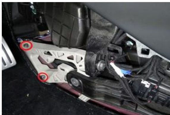
Figure 18. Releasing the toeboard bracket from the body
