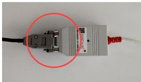
Figure 24. Connecting the EDR retrieval cable to the PCAN
