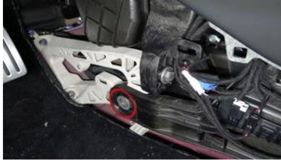
Figure 19. Releasing the toeboard bracket from the center console
