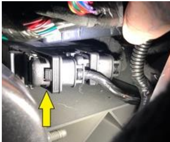
Figure 22. Disconnect the RCM connectors
