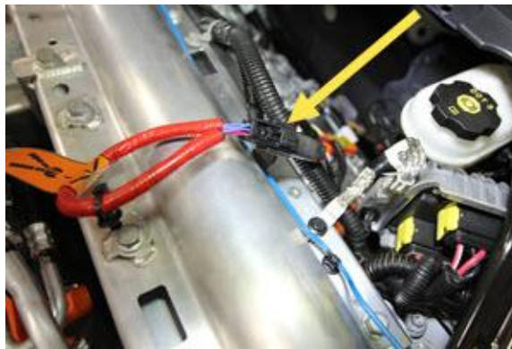
Figure 31. Disconnecting the First Responder Loop
