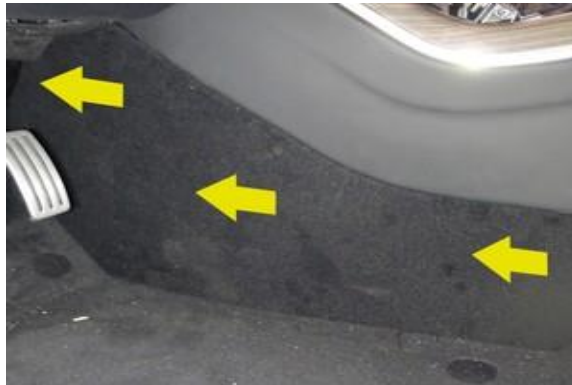
Figure 17. Removing the console side carpet
