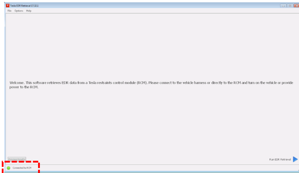
Figure 51. EDR program successful connection
