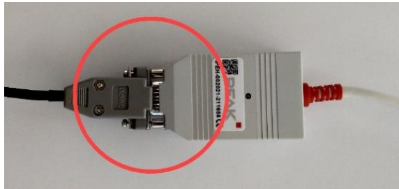
Figure 42. Connecting the EDR retrieval cable to the PCAN
