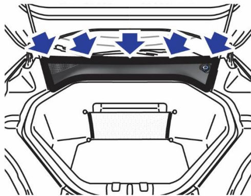
Figure 48. Removing the first responder access panel
