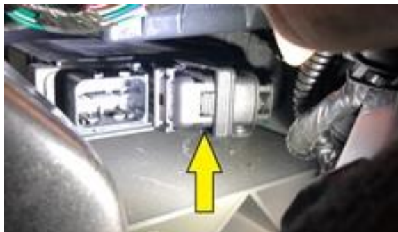
Figure 39. Disconnect the RCM connectors
