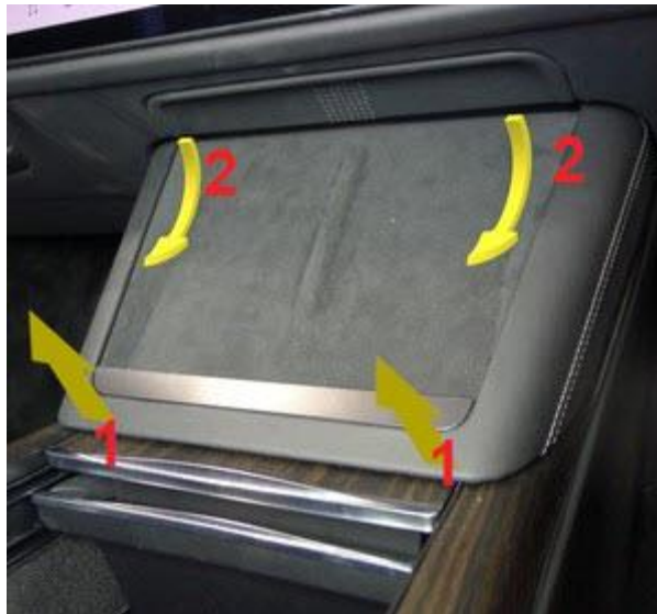
Figure 2. Releasing the phone dock
