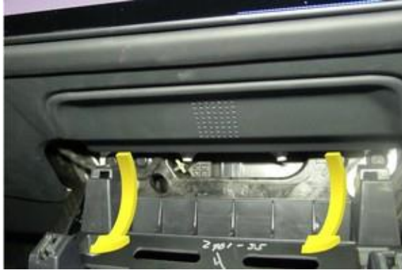
Figure 6. Removing the IP service panel
