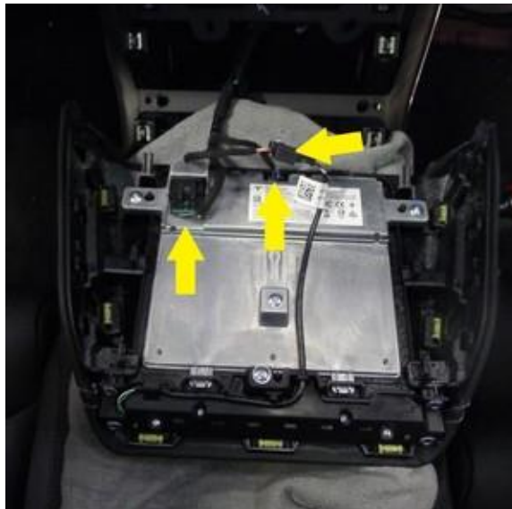
Figure 4. Releasing the phone dock connectors
