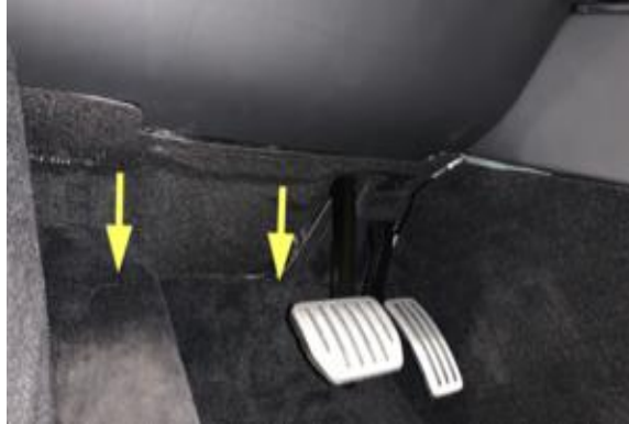
Figure 16. Removing the LH footwell cover
