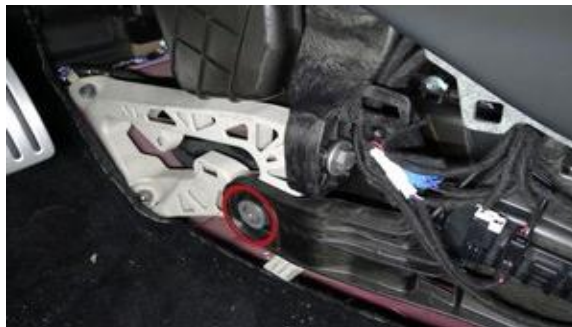
Figure 35. Releasing the toeboard bracket from the center console
