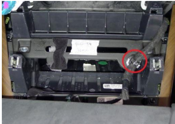
Figure 3. Releasing the phone dock wire clip
