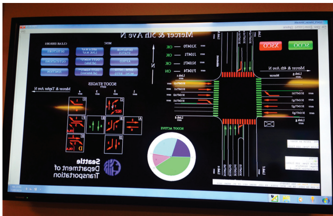
Figure 4: SCOOT in Action in SDOT's Transportation Operations Center
