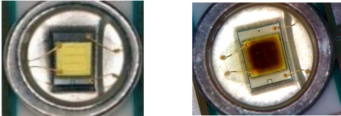
Figure 6: Examples of normal (left) and VOC degraded LED (right)
