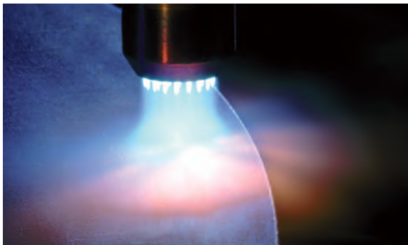
Figure 9. The application of preheat gases.
