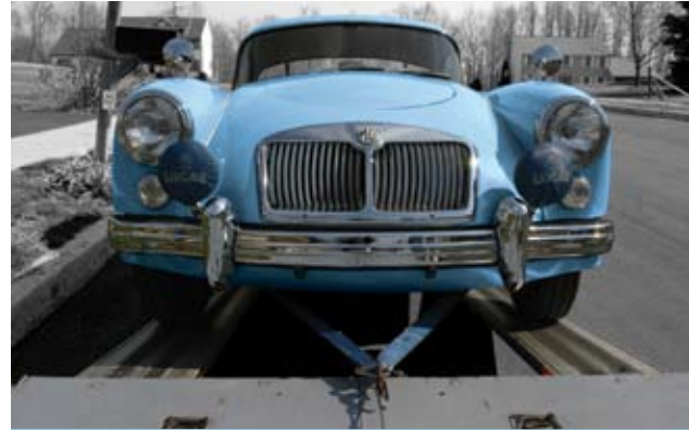
Loading a trailer alone is a lot easier when using a bridle harness and a winch. The combination allows you to inch the car up the ramps while ensuring it's properly aligned. Photo by Jay Texter
