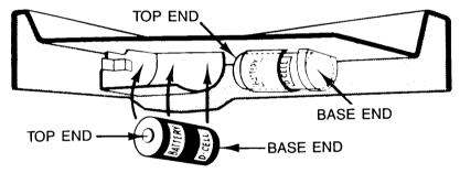
After the batteries are in place, test the "action" by touching the "SURGICAL" TWEEZERS to the metal edge of a "Cavity." This should make the "Nose" light up and the "Buzzer" sound. If Nose does not light, lift off Red Nose Cap and tighten bulb. To replace burned out or broken bulb, use only Type 14A, 2.5 volt screw bulbs (flashlight style bulb).
