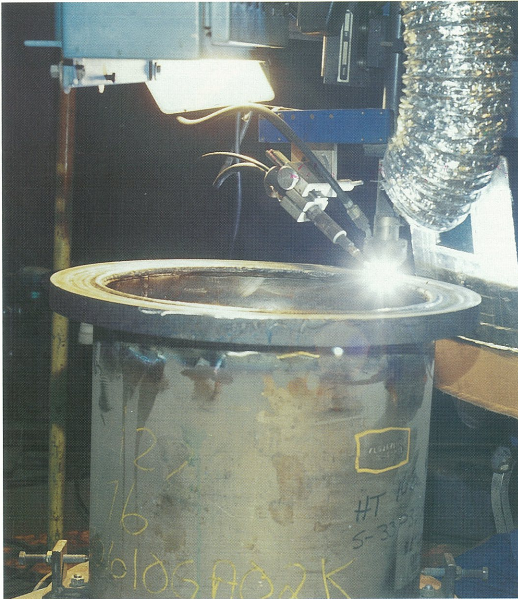
Figure 3.13—GTAW Cladding A Steel Flange with Copper-Nickel
