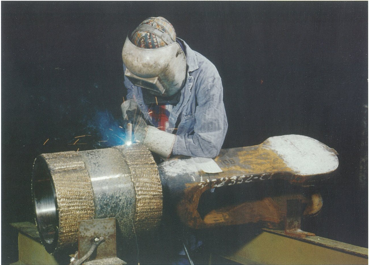
Figure 3.14—Surfacing a Mining Shovel Casting
