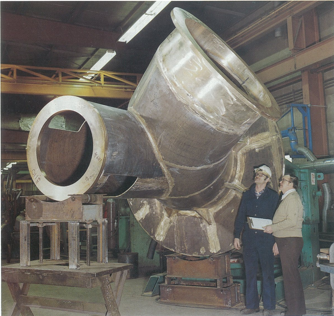
Figure 3.11—Pump Discharge Elbow Fabricated with Aluminum Bronze
