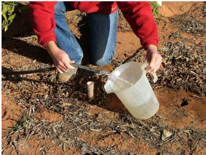
Figure 2. Measuring lateral discharge rates into a bucket
