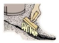
**FIG. 3** - Moisten the area to be repaired with cement adhesive or water.
