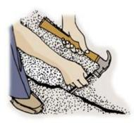
**FIG. 1** - Enlarge the crack with a cold chisel and a hammer before attempting to repair it.
