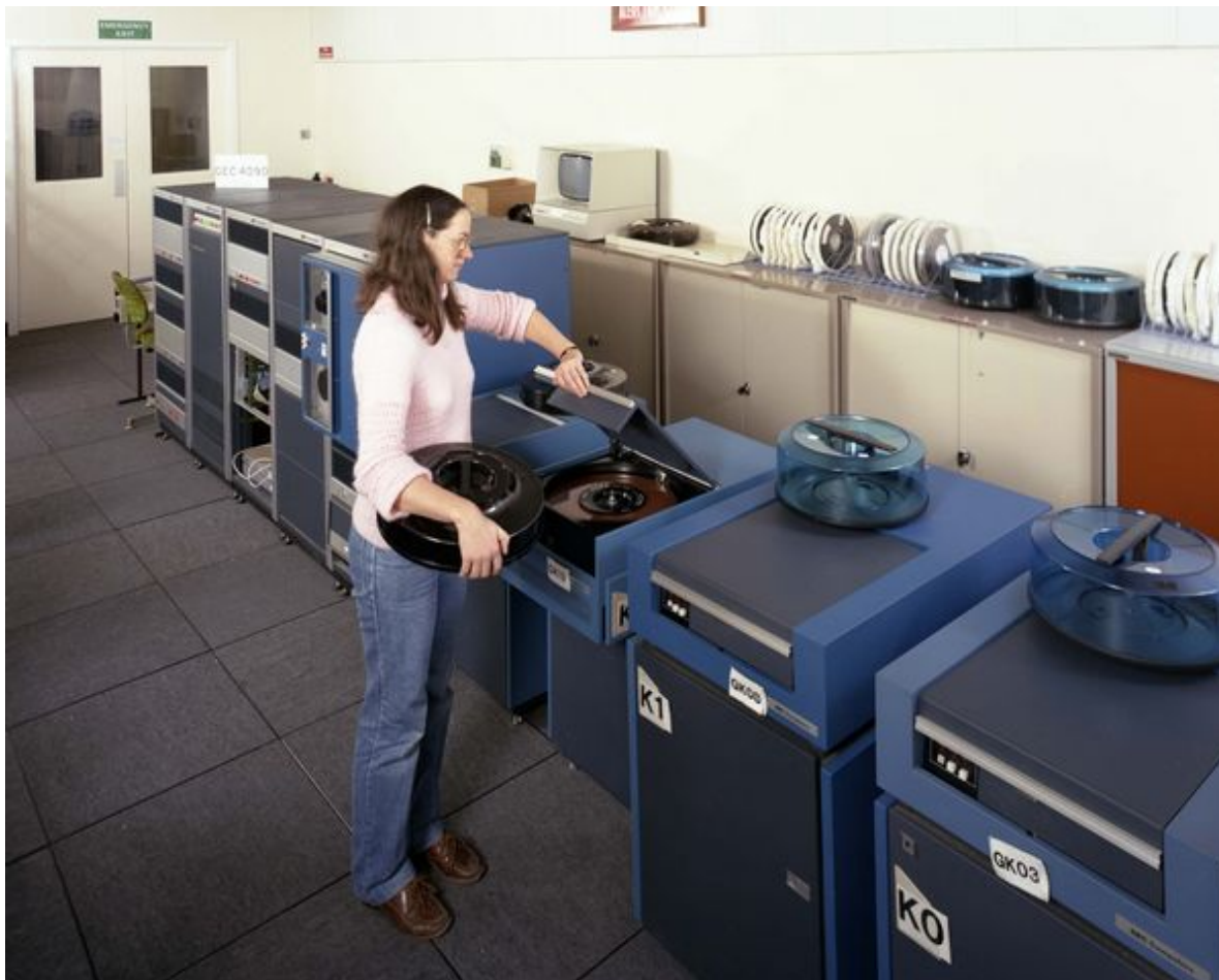
Informatics Machine Room in R1, June 1986, Shirley Wood and GEC 4090 System
