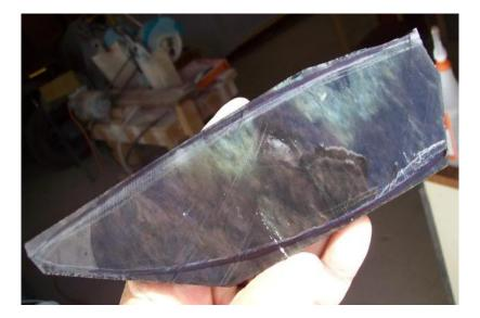
Take a slab, orient it the way you want, mark out the shape and trim with a tile saw. Closer triming here save diamonds later! I slab my own with an 18" Highland Park.
