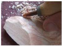
Using the side of the copper tip to trim the edge to shape, in a shearing motion.
