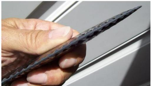
Back to the grinder (fine wheel) and grind down about 1/16 to 1/8" of the deltas on both sides, leaving a fairly sharp edge for the final retouch.
