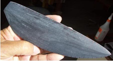
Grind out the shape then grind both faces into a convex shape. Leaving a median ridge down the middle helps the flakes treminate smoothly. I'm not always successful. Rough it out with the coarse wheel leaving about a 1/16" flat on the edge so you don't rip the edge off. Smooth it out removing all the grind scars with the fine wheel. Start with thicker slabs to allow for grinding removal.
