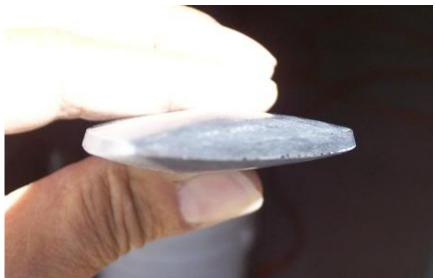
Using the fine wheel, bevel the edge at about 75 to 80 degrees. This edge should be straight with a sharp edge on the side to be flaked. This is your working edge for one face. Measure and mark, if you want to, the evenly spaced flake locations.
