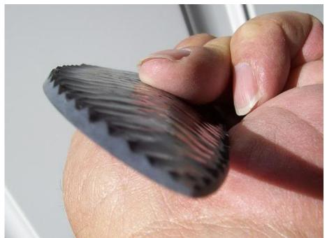
Back to the grinder (fine wheel) and bevel the working edge back the other way to flake the other
