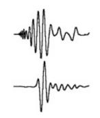
The key to Patriot's Radar system is its ability to transmit and receive pulses barely longer then single cycles at the transmit frequency. The first waveform shown here is a pulse generated by an earlier Patriot Design, based on "off the shelf" antenna technology. The waveform on the bottom was produced and received by Patriot's current Design.
