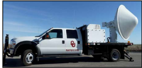
Figure 5. The University of Oklahoma's RaXPoI radar which scanned the El Reno tornado.
