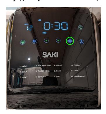
Set the timer for the **FIRST REST** setting by changing the arrows pointing up and down to **30** minutes.
