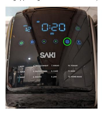
Set the timer for the **THIRD REST** setting by changing the arrows pointing up and down to **20** mins.
