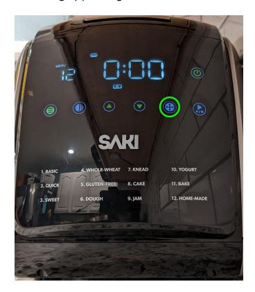
Set the timer for the **SECOND KNEAD** setting by changing the arrows pointing up and down to **0** mins.
