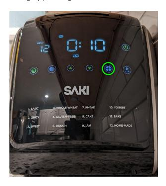
Set the timer for the **THIRD KNEAD** setting by changing the arrows pointing up and down to **10** mins.
