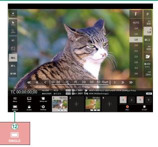
A 4-screen display button has been added. If this button is pressed, the screen display is divided into four parts to check the live views of multiple cameras at the same time.
