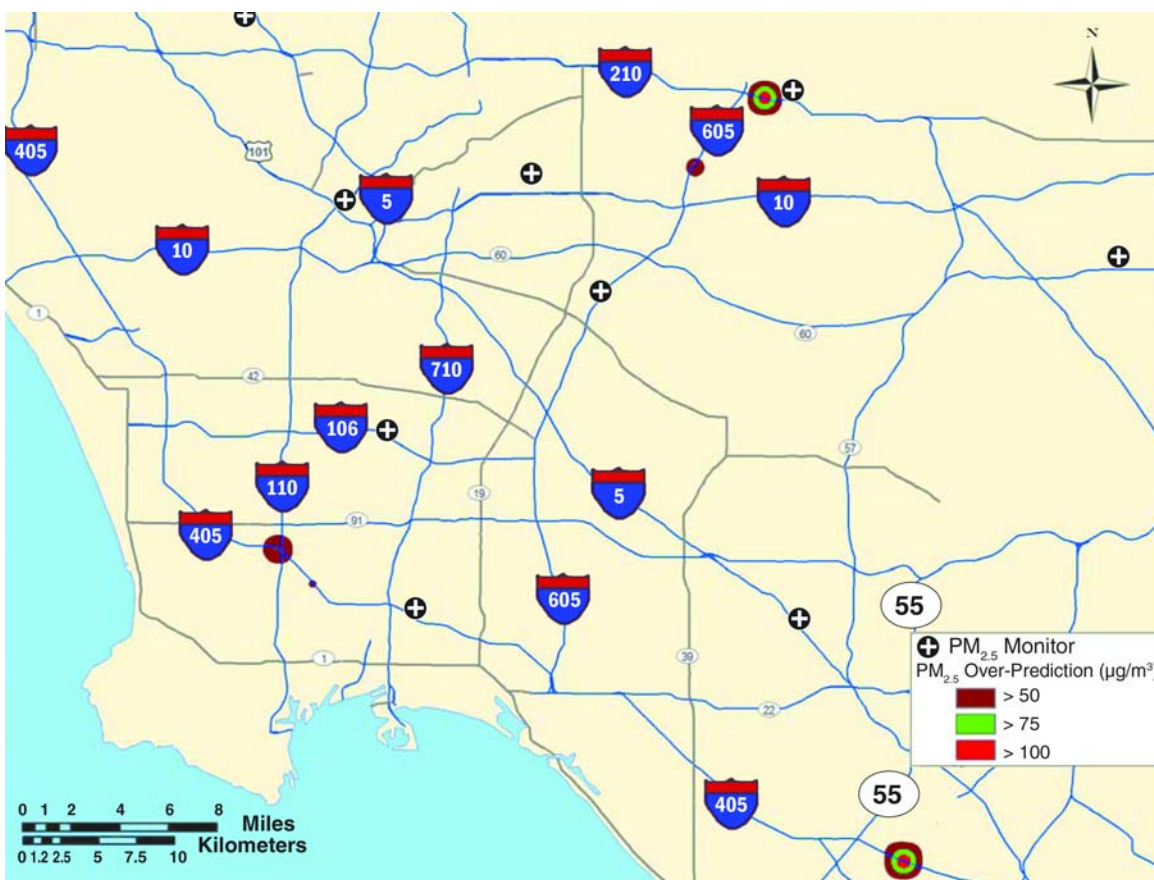
Figure 13. Map of over-predicted values from the LUR model, shown as > 50 , 75 , or 100 \mu\text{g}/\text{m}^3 higher than the measured value. Most over-predictions occurred at freeway intersections. \text{PM}_{2.5} monitor positions are marked with a +.
