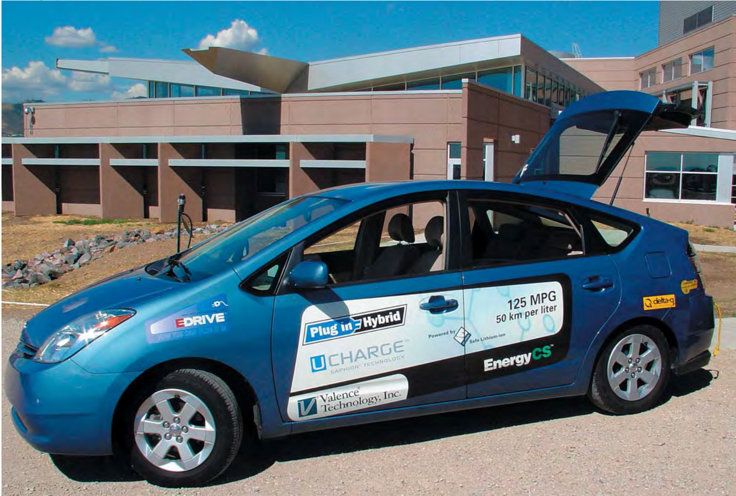
This Toyota Prius has been converted into a plug-in hybrid electric vehicle so that its electric battery can be recharged by plugging its cord into a standard 110-volt outlet. A computer inside the vehicle determines when it is most efficient for the vehicle to be fueled by electricity or by liquid fuel (either petroleum or biofuels).
