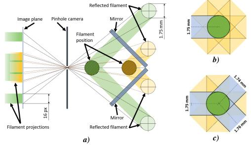
**Figure 4. Image acquisition scheme:** a) image acquisition based on the pinhole camera model; b) filament projection in the absence of mirrors; c) filament projection with two mirrors installed at 45-degree angles
