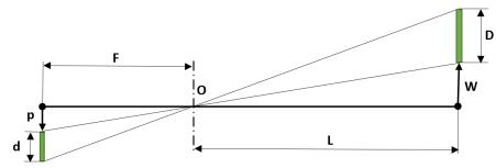
Figure 5. Pinhole camera model
