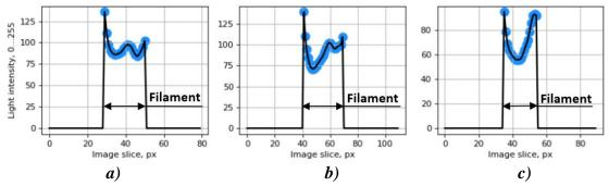
**Figure 8. Vertical slices of the segmented filament section:** a) upper mirror projection; b) main image; c) lower mirror projection.
