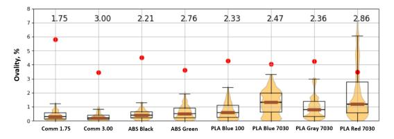
Figure 15. Distribution of ovality values obtained by optical diameter measurements with the camera. Red dots represent the maximum allowable ovality for each diameter.
