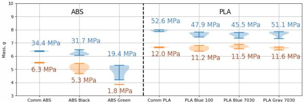
Figure 16. Mass distribution of the produced tensile bars (blue) and compression cylinders (orange) with indicated average tensile strength (blue) and compressive stress (orange) values.
