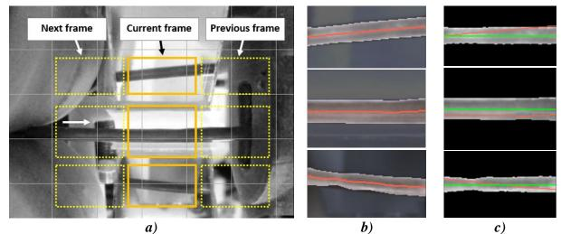
**Figure 6. Filament segmentation and diameter measurement procedure:** a) single camera frame; b) segmented filament; c) rectified regions reveal filament thickness and its surface structure based on light intensity. The red lines represent the detected filament centerlines, while the green ones represent their straightened counterparts, making it easier to concatenate adjacent texture sections together.
