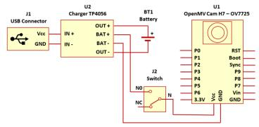
Figure 2. Wiring diagram
