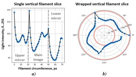
**Figure 9. Filament surface based on reflected light intensity:** a) a slice of a concatenated segmented filament image in a direction perpendicular to its length; b) cross-section of a wrapped pseudo-surface
