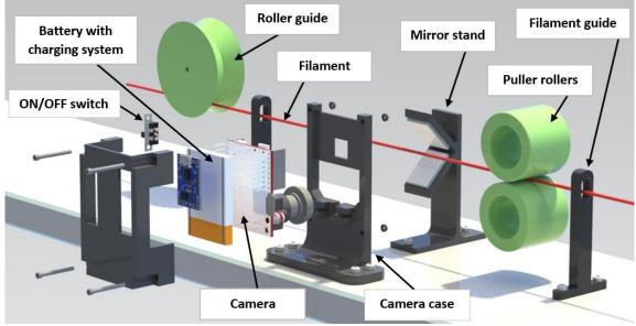
Figure 1. Schematic view of the open source single camera-based optical diameter measuring system
