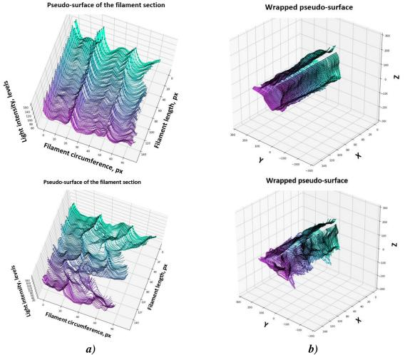
**Figure 10. Pseudo-surface of the filament section obtained in one image frame:** a) light intensity distribution over the entire surface of the filament section; b) wrapped pseudo-surface for the normal (top) and abnormal (bottom) sections of filament.
