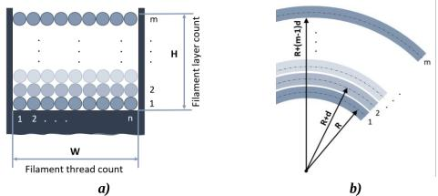
Figure 3. Spool winding diagram: a) schematic front view; b) schematic side view.
