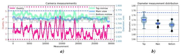
**Figure 13. Measuring the diameter of a commercial 1.75 mm filament:** a) diameter and ovality measurements during the winding process; b) diameter distributions for the main image and upper and lower mirror reflections. Dashed and dotted lines represent the manufacturer's declared diameter and ovality tolerance limits, respectively.
