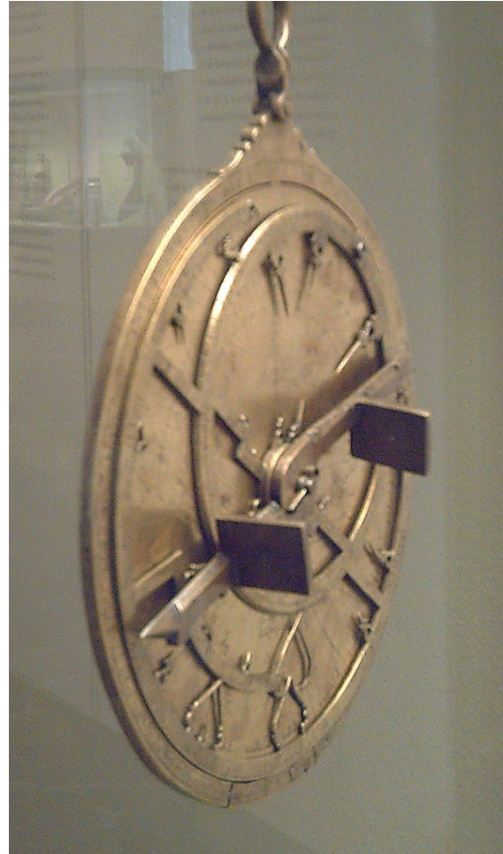
Figure 29: The sighting vanes on the alidade
