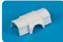
Cable Inlet/Outlet Takes cables in or out of a 30x15mm Mini Trunking installation. Use between lengths on straight runs
