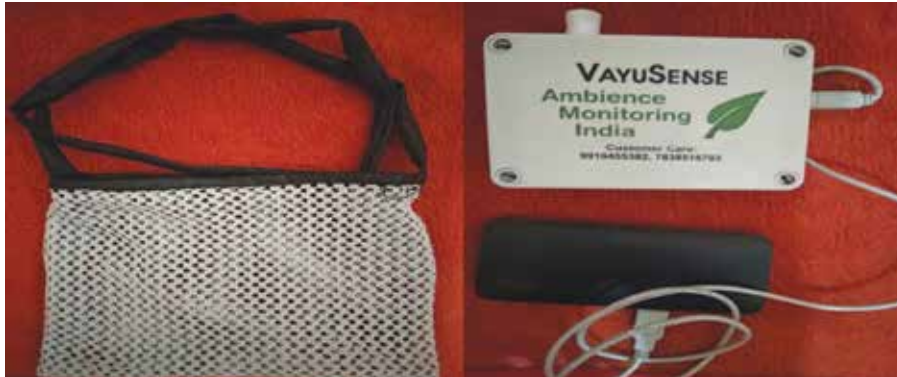
Air pollution monitoring device with power source and sling bag
