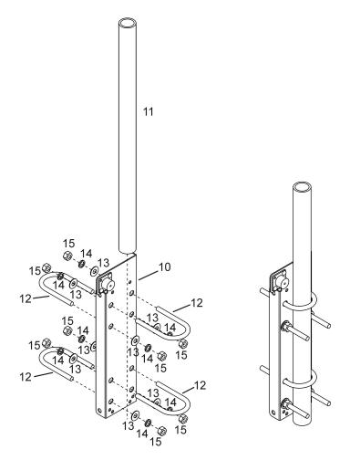
Assemble the base using the Base Plate (10), four U-Bolts (12), eight  $\frac{1}{4}$ " flat washers (13), eight  $\frac{1}{4}$ " lock washers (14), and eight  $\frac{1}{4}$ -20 nuts. Loosely attach the U-Bolts then slide the fiberglass base insulator (11) into the U-Bolts as shown in the picture and tighten up the U-Bolts holding the fiberglass base insulator.
