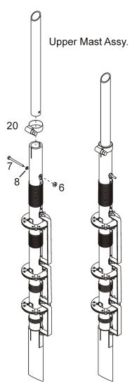
Slip the upper mast assembly and the 1.25" hose clamp (20) into the loading coil assembly and align the holes then slide the 6-32x1.5 SS screw (7) and #6 lockwasher (8) through the holes and the solder lug. Attach the 6-34 KEP nut (6) to the screw and tighten down. Tighten the hose clamp.
