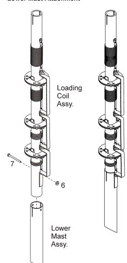
Attach the lower mast assembly to the loading coil assembly using 6-32x1.5 SS screw (7) and 6-32 KEP nut (6). Slide the mast assembly over the fiberglass tube and align the hole in the aluminum tube with the fiberglass tube. Slide the screw through the holes and attach the nut. The solder lug will be between the aluminum tube and the jumper bracket. Tighten the nut and screw.
