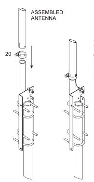
Slide the assembled antenna and the 1.25" hose clamp (20) onto the fiberglass tube. Place the wire from the coax connector under the hose clamp between the clamp and the antenna mast. Raise the antenna mast up so it is about 1 inch above the mounting base plate then tighten the hose clamp to hold the antenna and wire in place on the base. Make sure the wire or the mast section does not touch the base plate.
