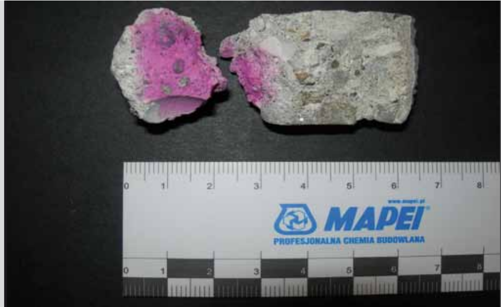
photo 6 Colour test using phenolphthalein
