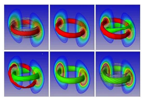
FIG. 13. Nonlinear simulation of internal magnetic reconnection event in the National Spherical Torus Experiment.
