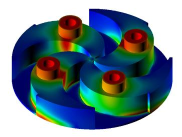
FIG. 4a (left). Geometric model of an optimized linear collider accelerating cavity design based on an unstructured grid and partitioned for load balancing. FIG. 4b (right). Results of a parallel simulation showing the current density, indicated by color, in a preliminary design for a PSI cyclotron project.
