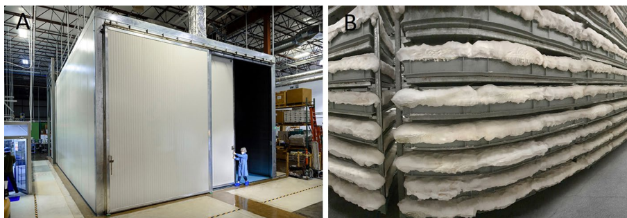
Fig. 7 A. Incubation chamber for large scale production ©Ecovative, B. vertical farming of aerial mycelium foam ©Bolt Threads
