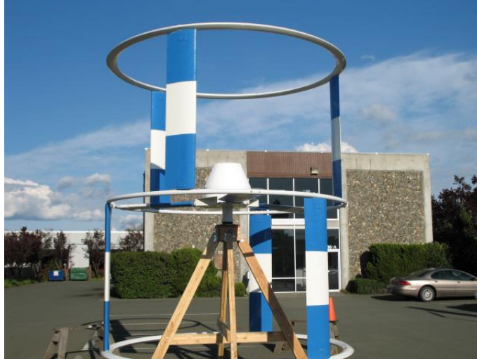
Figure 3. Experimental concept for a vertical sail wind machine with a 3 kW rated output.
