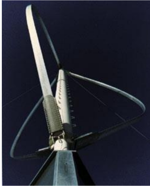
Figure 6. Blade end attachments in a Darrieus wind turbine.
