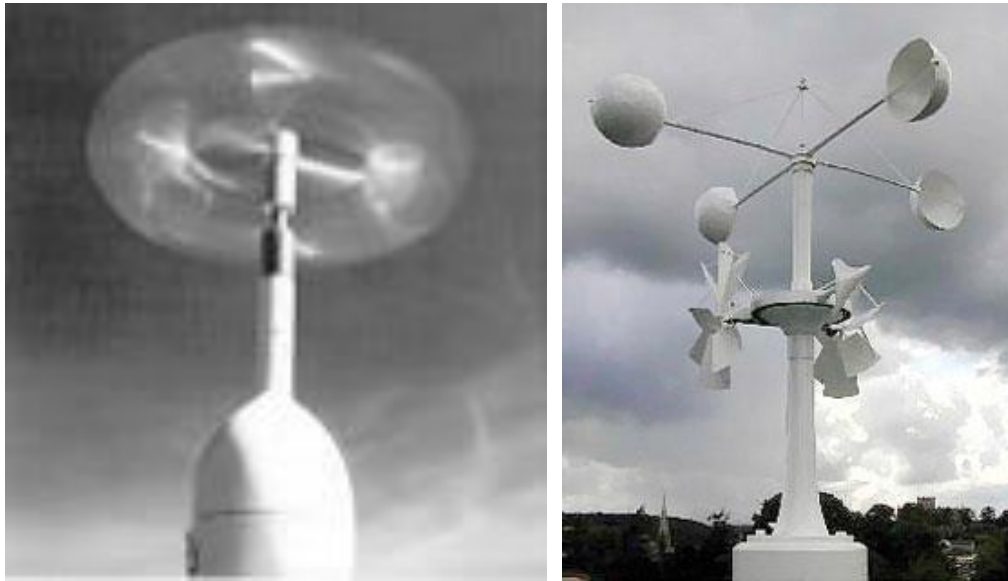
Figure 9. Rotating cup anemometer and drag cup wind turbine.
