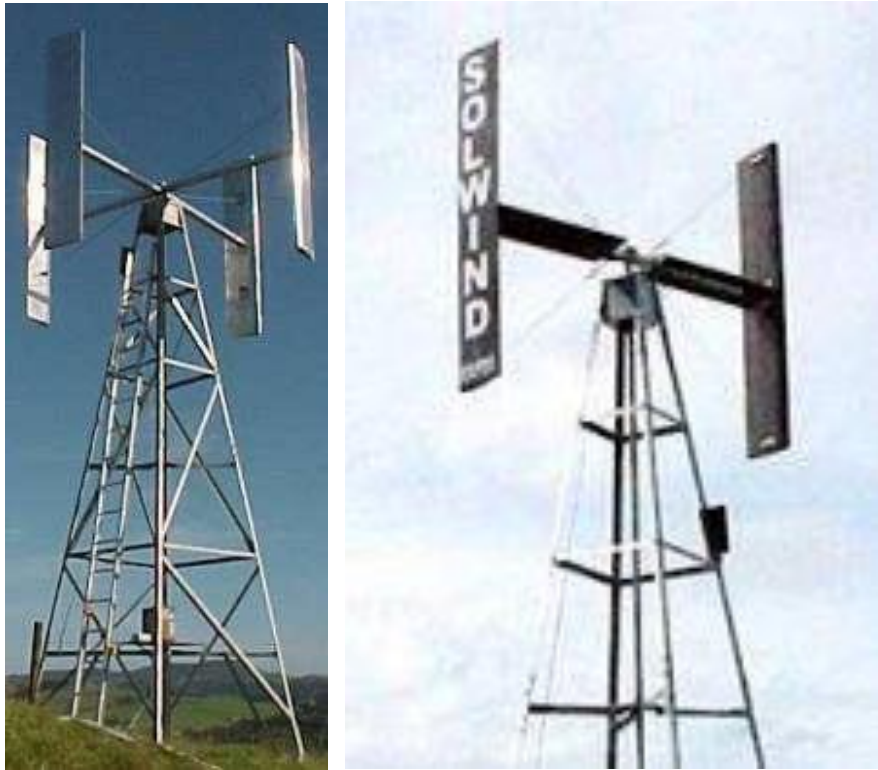
Figure 16. Two and four rotor blades vertical wind generators.
