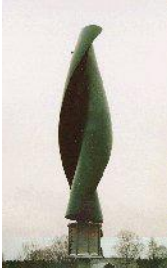
Figure 26. Helical wind turbine with generator at its base.
