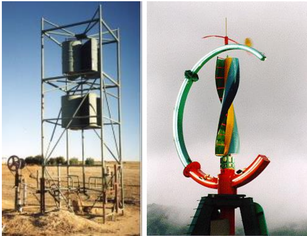
Figure 10. Evolution of the Savonius design for water pumping from half drums into the fluted spiral bladed design.
