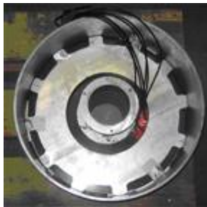
Figure 32. Air core generator used with the Windspire turbine.
