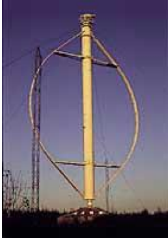
Figure 11. Eole C 4.2 MW Darrieus vertical axis wind turbine, Cap Chat, Québec, Canada.
