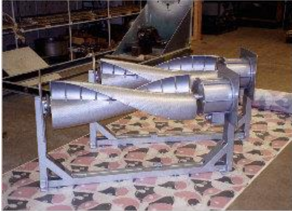
Figure 27. Manufacturing of helical wind blades. The generator is at right.
